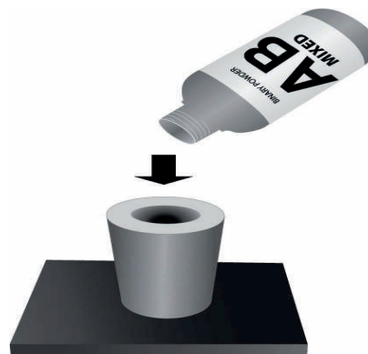
Loading Binary Powders into hardware
