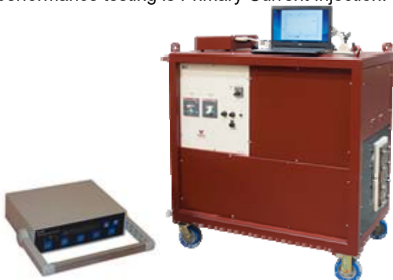
Figure 1 - Eaton MTK200 Trip Unit Test Kit for Secondary Current Injection
