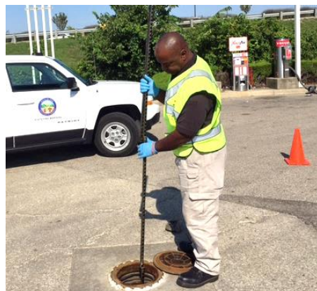
Fig. 5 - manual tank gauging (MTG)
