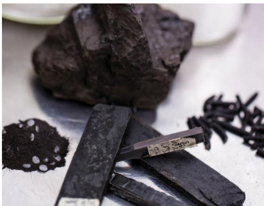
Ohio University coal plastic composite materials; including source coal, compounded coal plastic composite material, and specimens for testing.
