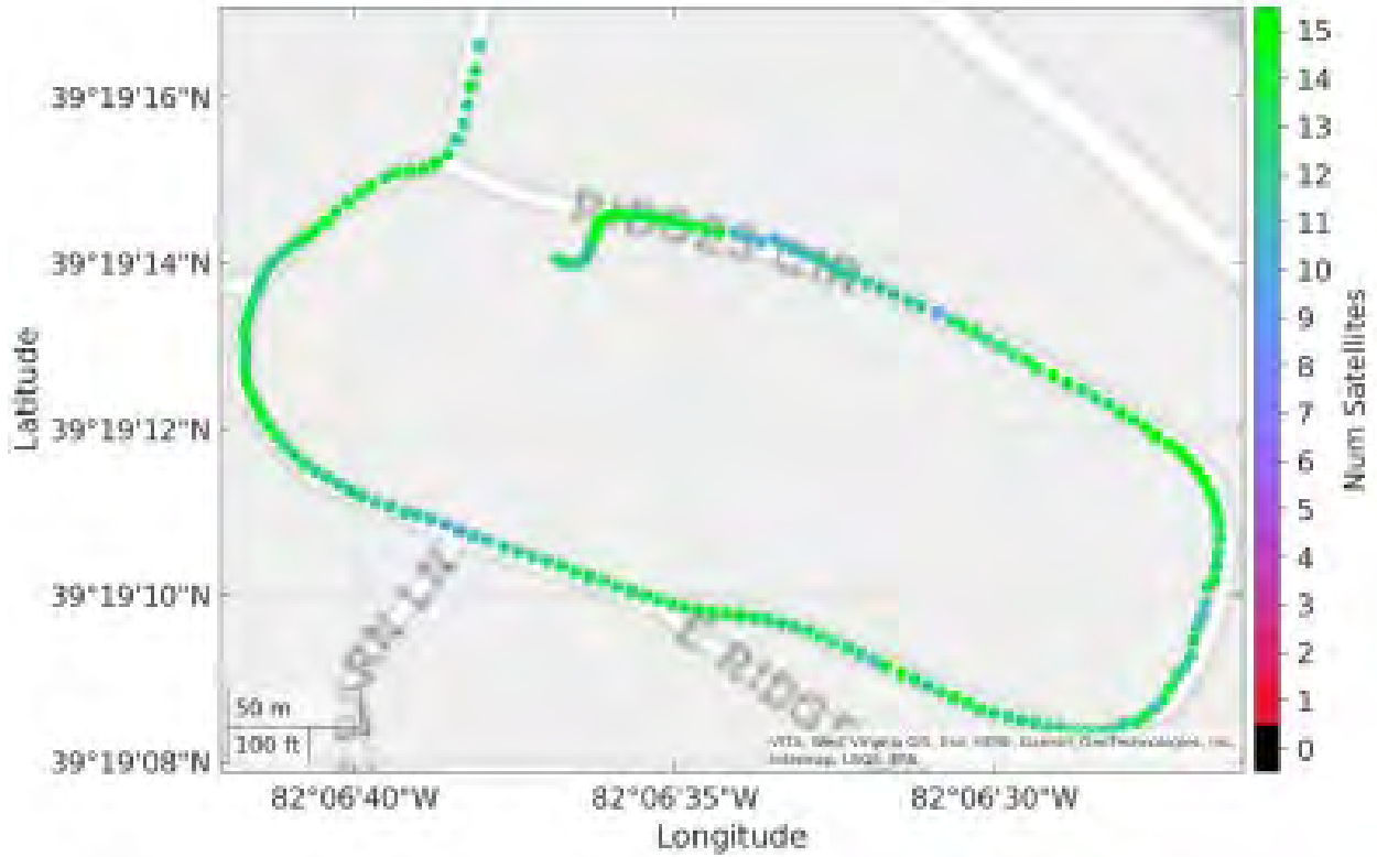
Figure 19. GPS Coordinates of the van drive laid over the Mandli map with the number of received satellite signals.
