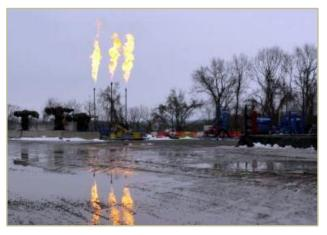
Example of a temporary flare system during well production testing after drilling is completed. Ohio EPA file photo
