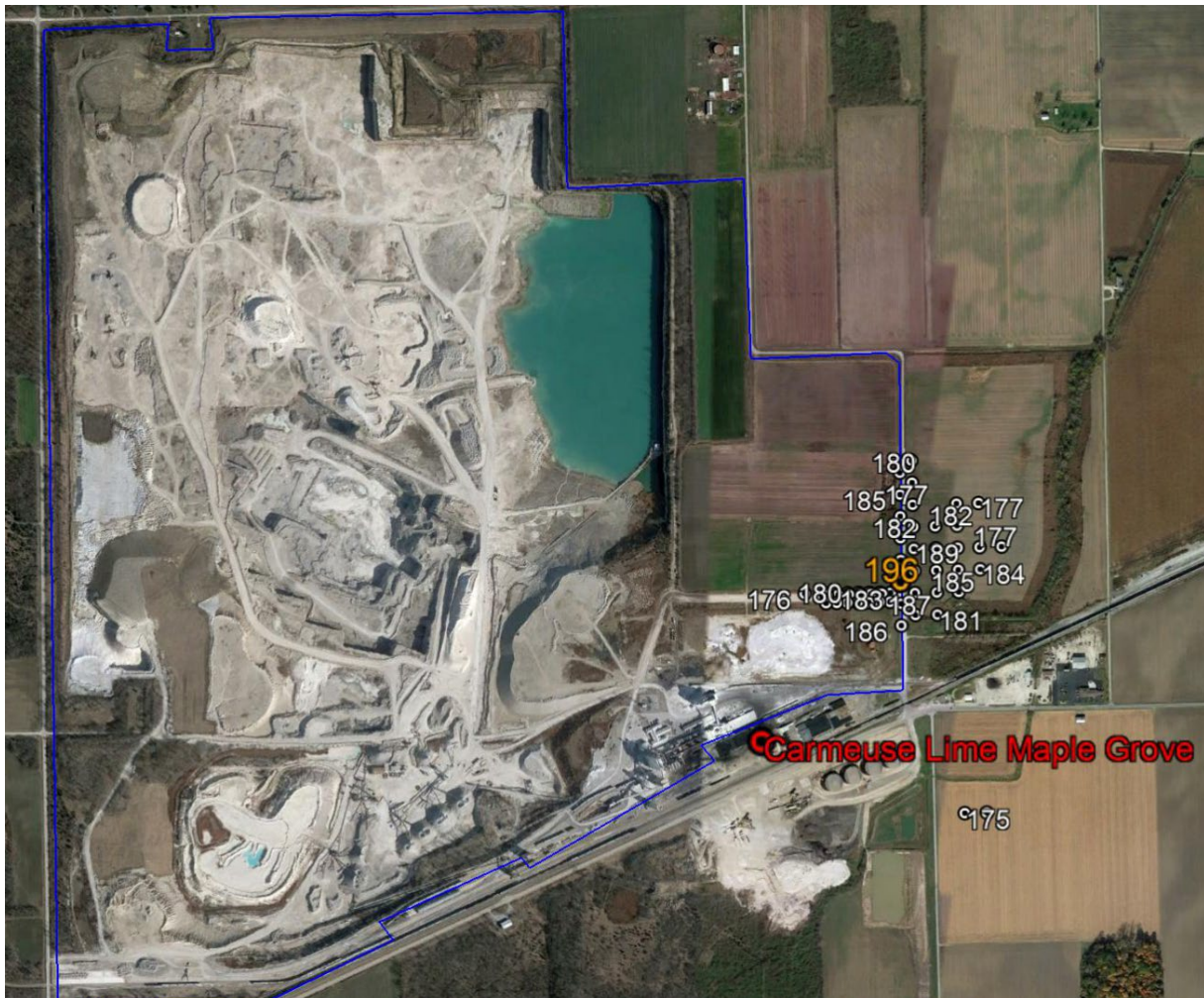
Figure A5: Compliant Emissions Scenario maximum SO 2 impacts, Carmeuse Lime Maple Grove and WIN Waste Innovations of Seneca County, 2019-2023. Concentrations in µg/m 3 , including background.
