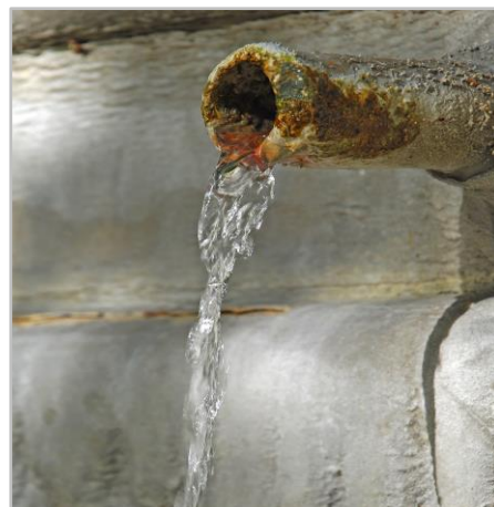
Figure 3. Water pipe that has rusted due to oxidation processes.
