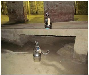
Collecting an indoor air sample and a sub-slab sample in the basement of a building
