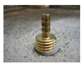
A close-up view of a sub-slab sample port.
