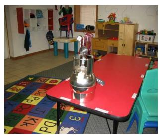
Sample canister collecting indoor air for analysis.
