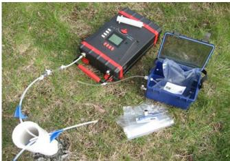
The photos above show different methods for collecting an air sample from a soil gas sampling system. The tubing shown in the photos are set at different depths below ground surface in order to evaluate the actual migration of the soil gas.
