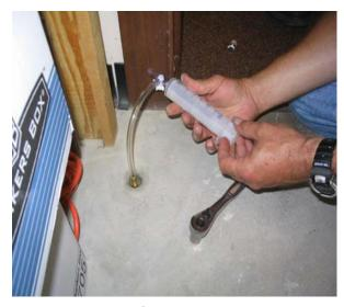
Collecting a gas sample from a sub-slab sample port.
