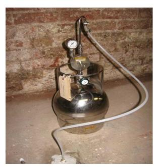
Collecting a sub-slab gas sample into a canister for laboratory analysis.
