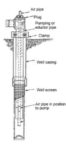
**Figure 8.2: Two pipe air-lift system** (Source: "Monitoring Well Development" by T.E. Gass. *Water Well Journal*, Vol. 40, No. 1, p. 54 (Figure 4). 1986. Reprinted from Water Well Journal with Permission from National Ground Water Association. Copyright 1986).
