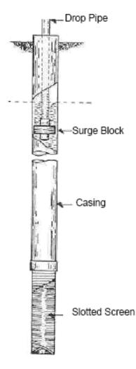
**Figure 8.1 Development with a surge block** (Source: "Monitoring Well Development" by T.E. Gass. *Water Well Journal*, Vol. 40, No. 1, p. 53 (Figure 1). 1986. Reprinted from Water Well Journal with permission from National Ground Water Association. Copyright 1986).
