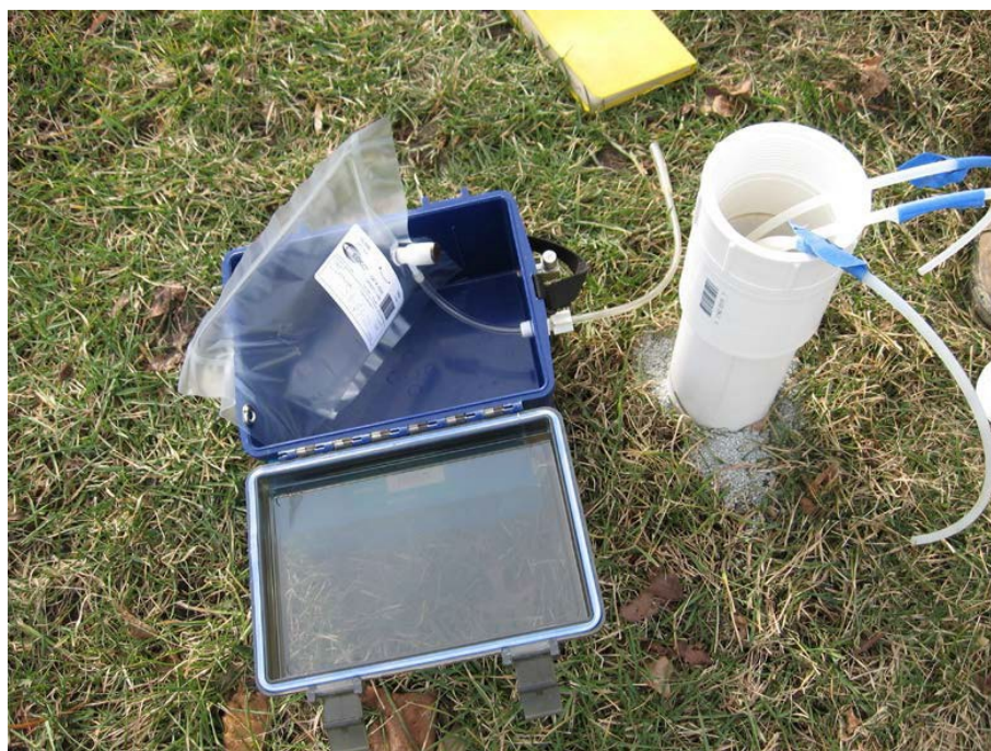
Semi-permanent soil gas probe location with multi-depth implants. The lung box sampler is used to collect soil gas samples using 1-liter Tedlar® bags. Note that each tube is labeled with the sampling depth; the PVC pipe is used to protect the soil gas tubing.
