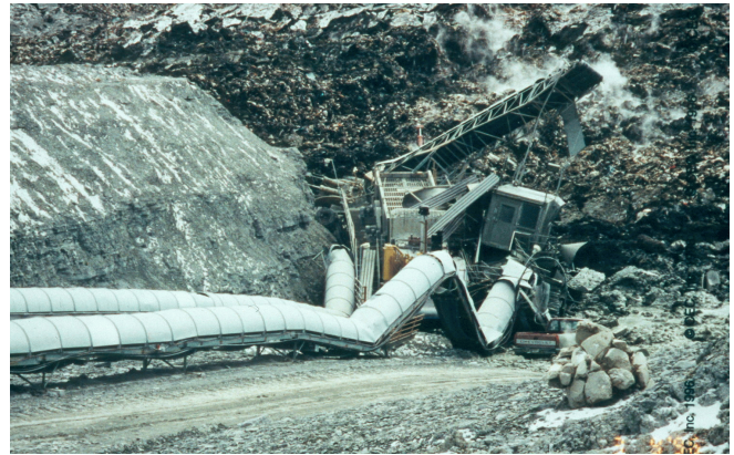
Figure 8-4, A sliding mass of waste is capable of producing enormous force as is demonstrated in this picture of mining and earthmoving equipment that were crushed by a large waste failure at an Ohio landfill. Photo courtesy of CEC, Inc.
