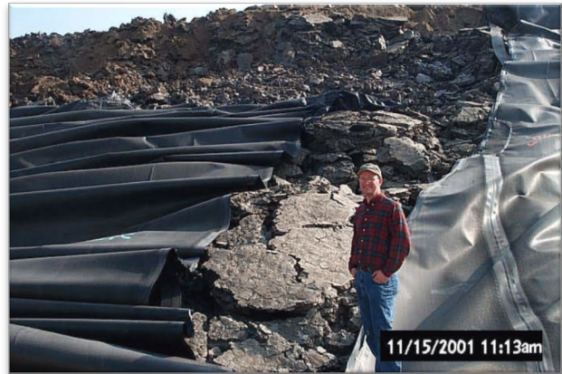
Figure 9-3. A translational failure through RSL at an Ohio landfill triggered by filling granular drainage material down slope.
