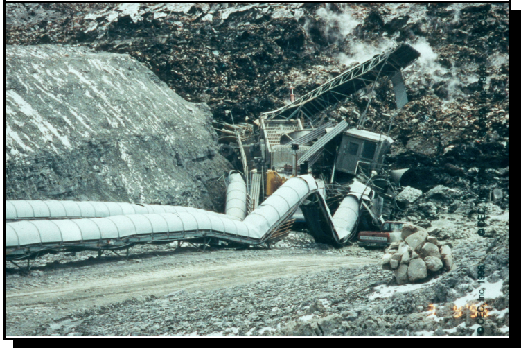
Figure 8-1 A sliding mass of waste is capable of producing enormous force as is demonstrated in this picture of mining and earthmoving equipment that were crushed by a large waste failure at an Ohio landfill. Photo courtesy of CEC, Inc.
