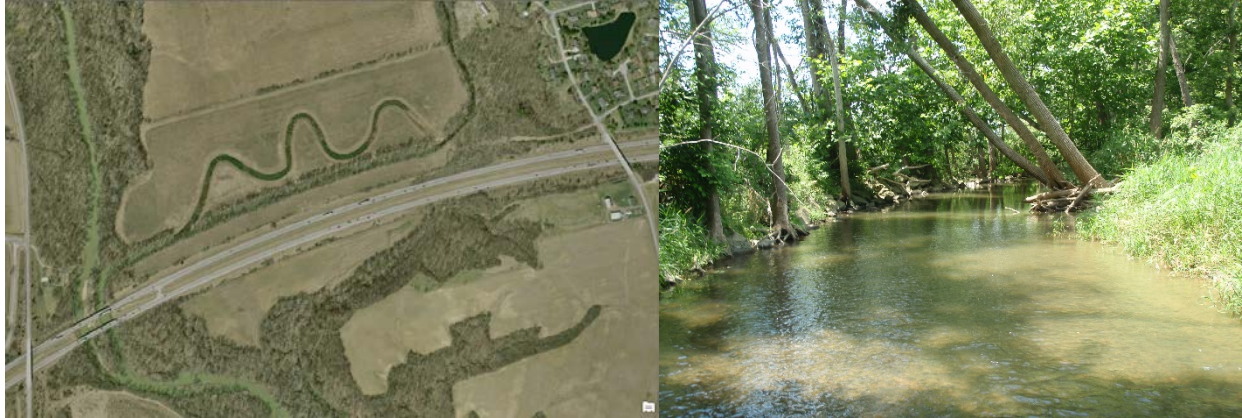
Figure 45. Constructed meandering channel near the mouth of Hellbranch Run with its confluence with Big Darby Creek (left). View on right shows older straightened and entrenched channel with sand/gravel bar covered in grass that blocks flow into new constructed channel at ~ RM 0.7-0.65. 2014.
