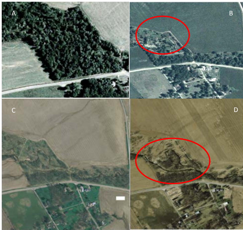
Figure 86. Historical imagery from lower Spain Creek. A) 2004, B) 2005, C) 2007, D) 2014. Note: 1) substantial riparian removal from the lower reaches of Spain Creek since 2004 and 2) construction of new, armored channel located to the south of the natural channel since 2004.
