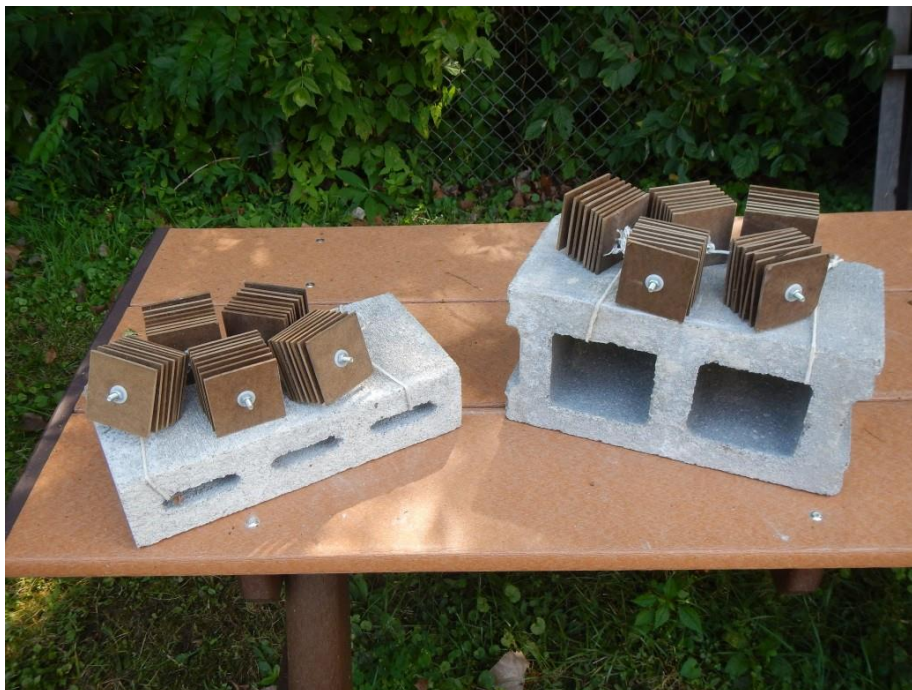
Figure 2 Configuration of artificial substrate samplers on cement block anchors used by the Ohio EPA to collect quantitative macroinvertebrate collections from small streams (left) and large rivers (right).
