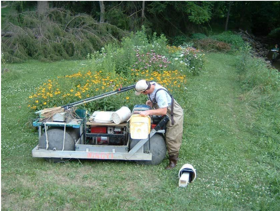
Figure 9 Side view of Rollerbeast with shelves and push-bar. Live well is adjacent to generator in the middle.
