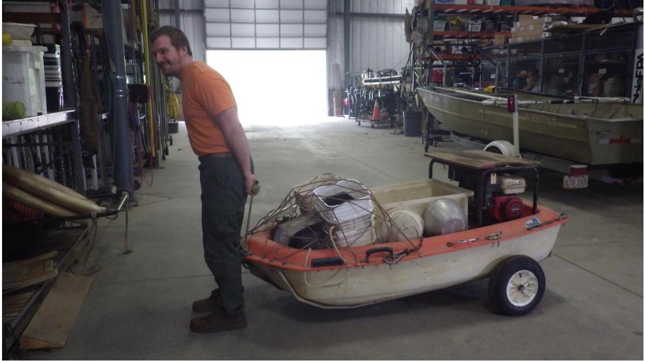
Figure 8 Sportyak with attached rear axle and wheels.
