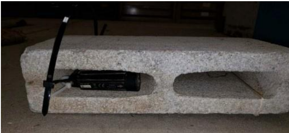
Figure 1. Temperature Logger Affixed to a Cinder Block
