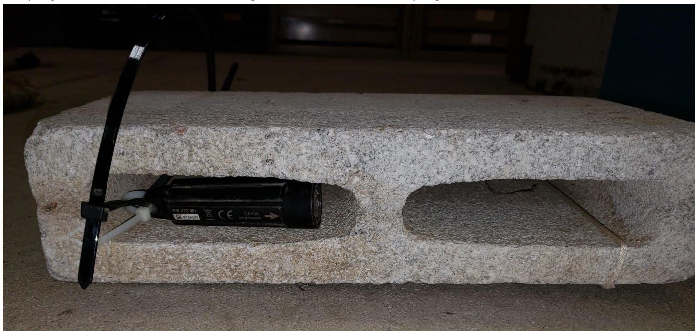
Figure 1. Temperature Logger Affixed to a Cinder Block
