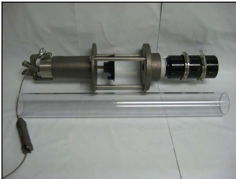
Figure 1. Picture of a modified K-B Corer with cable and messenger attached and a Polycarbonate core tube in the foreground.
