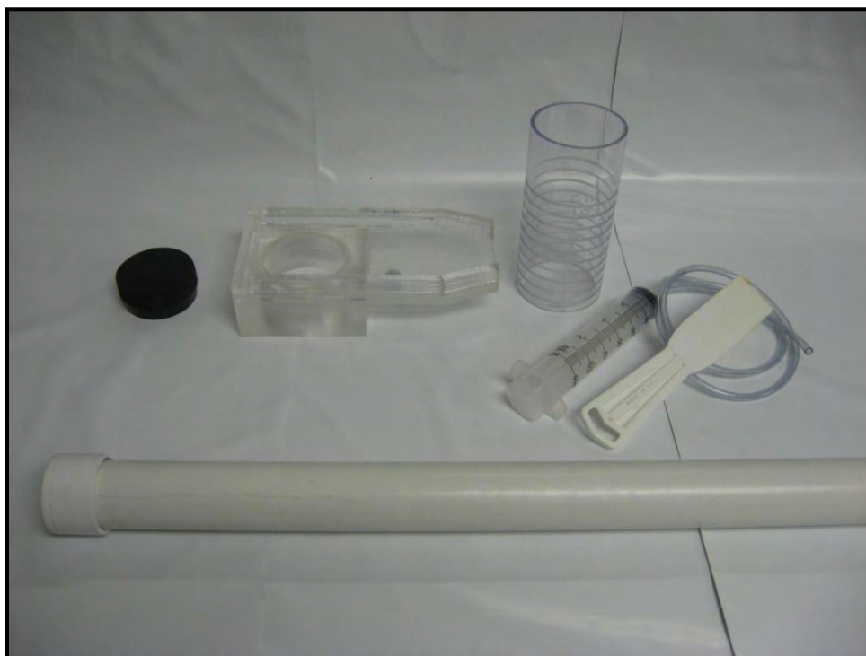
Figure 2. Picture of the core sectioning apparatus, with clockwise from upper left a rubber stopper, Plexiglas stage, metered sectioning tube, syringe with siphon tube, putty knife and PVC extruder.
