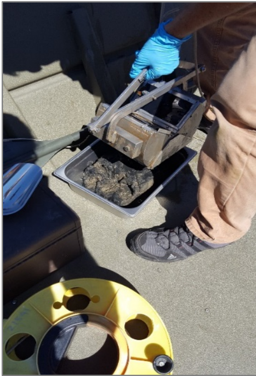
Figure 6. Use of a Petite Ponar dredge for lake sediment sample collection.
