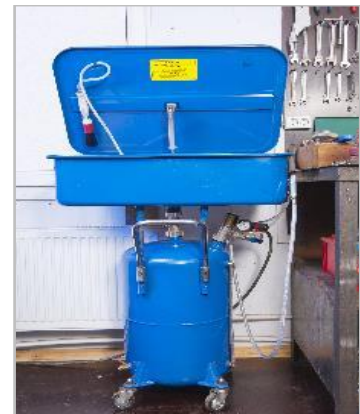
Some equipment, like small parts washers, may be exempt from air permitting.
