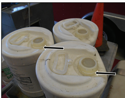
Breaks in lid ring seal as an indication that the cap has been potentially opened.
