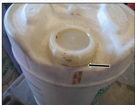
Worn/broken and misaligned tape seal as an indication that the cap has been potentially opened.
