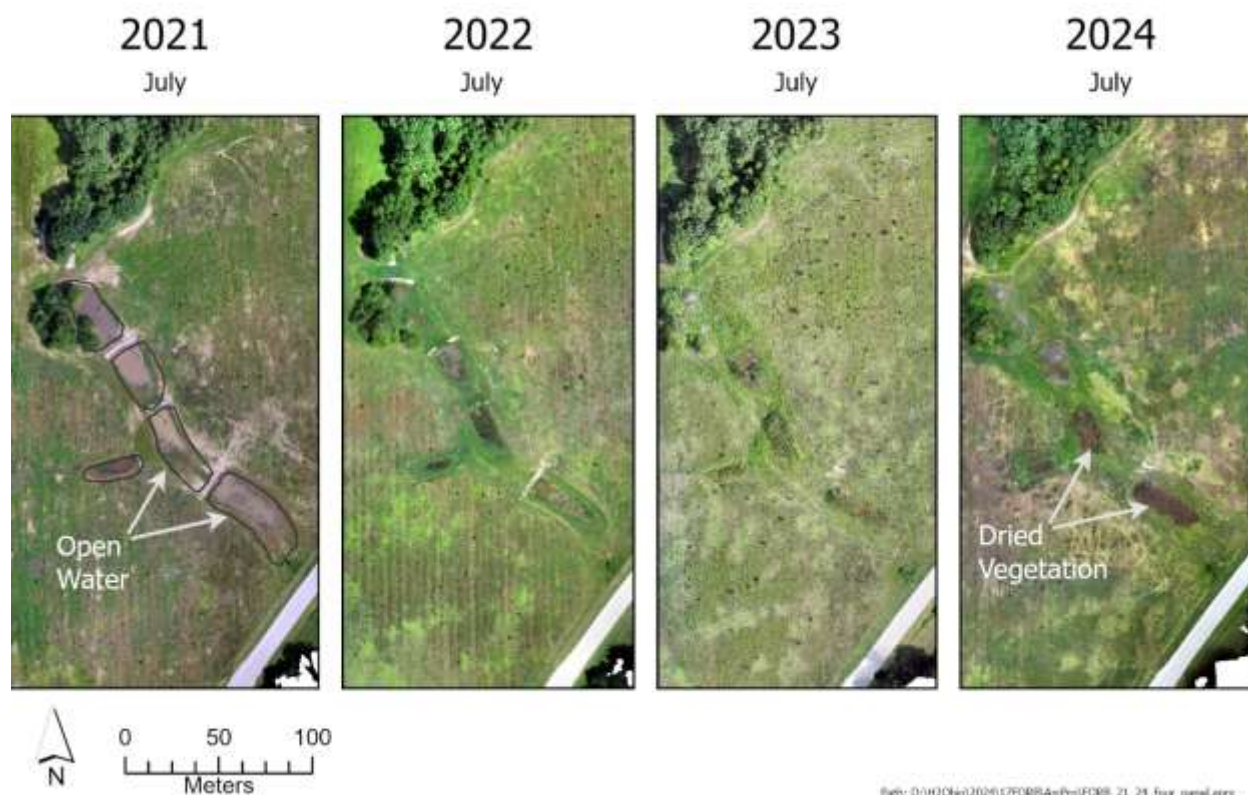
Figure 4. Unmanned aerial vehicle (UAV) images from Forder Bridge Floodplain Restoration Project in July 2021–2024 show pool extent and the effects of different water availability. In the wetter years of 2021 and 2022, larger areas of open water in treatment train pools are visible.
