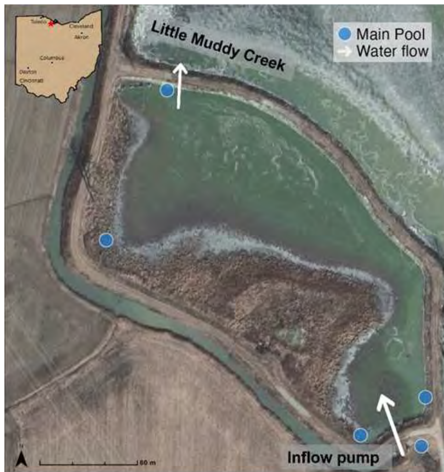
Figure 265. Aerial image showing surface water flow and sampling locations for the Buehler Farms Treatment Wetland Project. Blue arrows indicate direction of surface water flow. Dots
