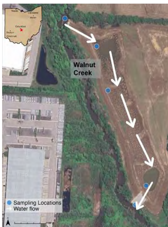
Figure 240. Aerial image showing surface water flow and sampling locations for the Walnut Creek Treatment Wetland Restoration Project. Blue arrows indicate direction of surface water flow. Dots represent geographic base crew sampling locations, which are grouped by Project features (fill color) where relevant. Text annotations provide additional context about the Project's watershed connection or other important features.
