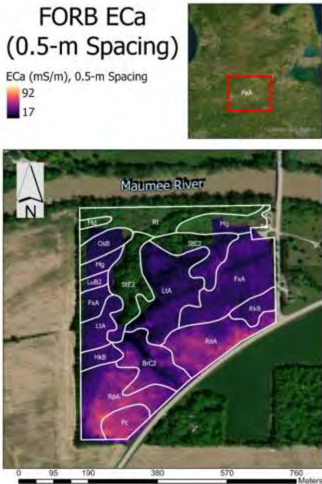
Figure 314. ECa data (0.5-m spacing) with NRCS Web Soil Survey soil zones overlayed over top.
