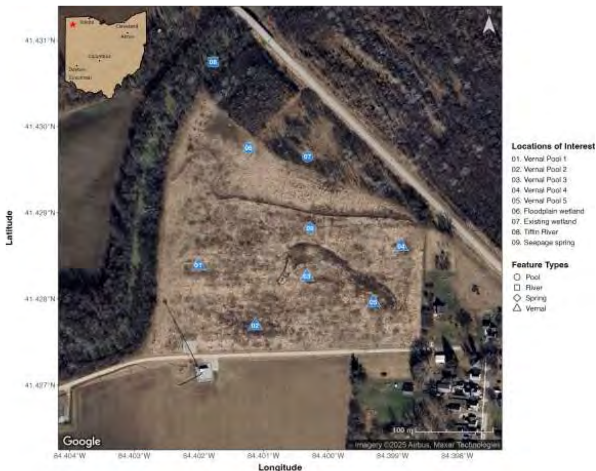
Figure 202. Aerial image of approximate locations of interest for water and soil sampling and discrete manual measurements of water depth and physicochemical parameters at The Weisgerber-Pohlman Nature Preserve Restoration Project during water year 2024 (Oct 1, 2023–Sep 30, 2024). The legend provides the name of each sampling point. Different shapes denote the types of wetland features represented by the locations of interest. If present, different colors
