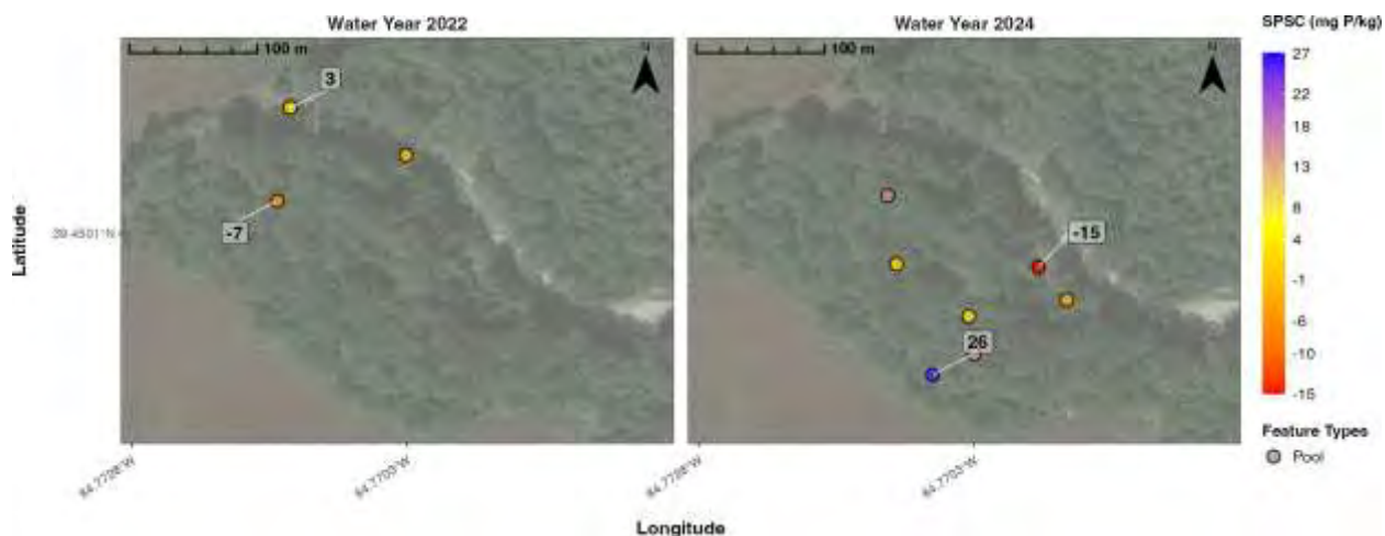
Figure 215. Soil Phosphate Sorption Capacity (SPSC) throughout the Indian Creek-Hoffmann Wetland and Stream Restoration Project. Each point denotes a soil sample (0–5 cm) and different shapes indicate the wetland feature type, as shown in the legend. Colors indicate the SPSC value of each sample relative to the overall range of values observed at the wetland project, as shown in the color bar. Each panel shows the soil samples collected during a respective water year (Oct 1–Sep 30), along with the minimum and maximum SPSC values observed during a given water year. Negative SPSC values indicate the potential for soils to release phosphate, while positive values indicate soils have capacity to sorb phosphate, based on Mehlich-3 extractions of phosphate, iron, and aluminum.
