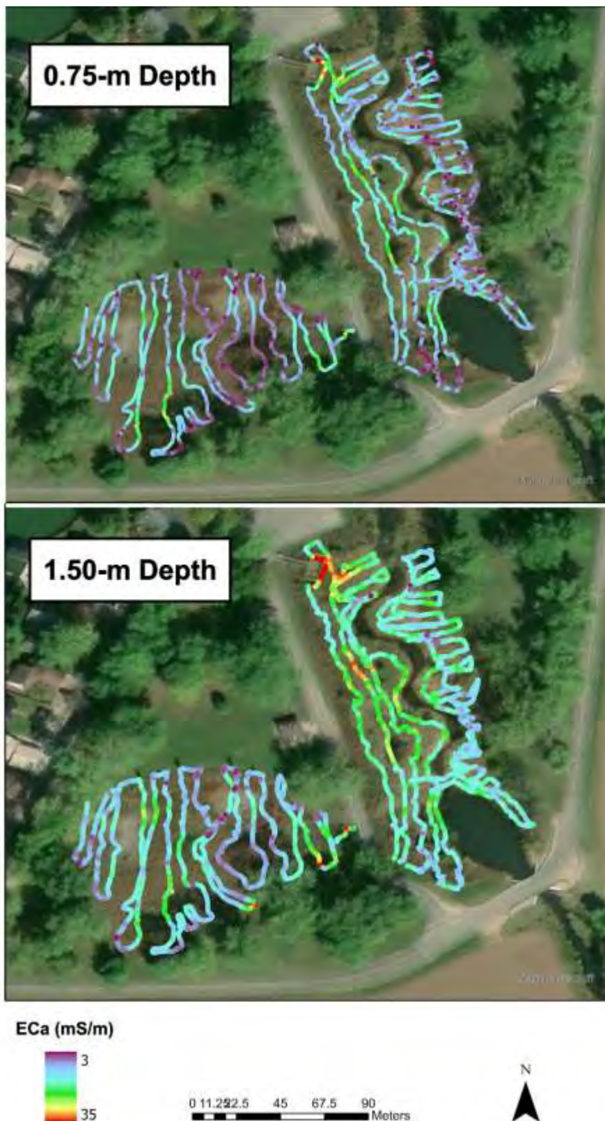
Figure 30. Apparent bulk soil electrical conductivity (ECa) at Brooks Park Wetland Creation & Water Quality Initiative Project in October 2024 for the (top) 0.75-m depth and (bottom) 1.5-m depth of investigation.
