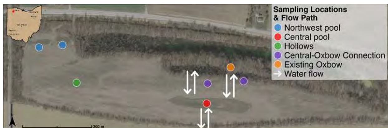
Figure 165. Aerial image showing surface water flow and sampling locations for the Maumee River Floodplain: H2Ohio Restoration Project. Blue arrows indicate direction of surface water flow. Dots represent geographic base crew sampling locations, which are grouped by Project features (fill color) where relevant. Text annotations provide additional context about the Project's watershed connection or other important features.
