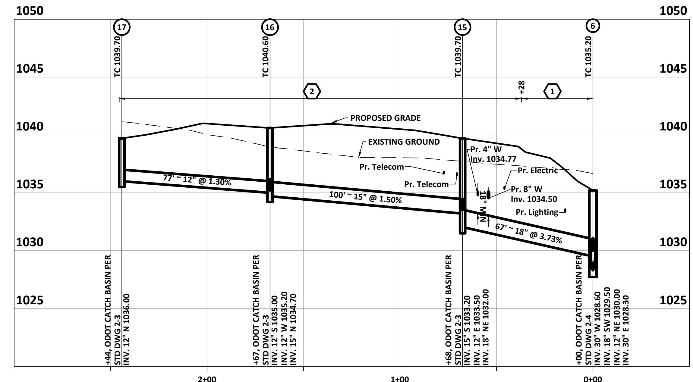
STORM SEWER 6 TO 17 PROFILE SCALE: 1"=30' HORIZ. 1"=5' VERT.
