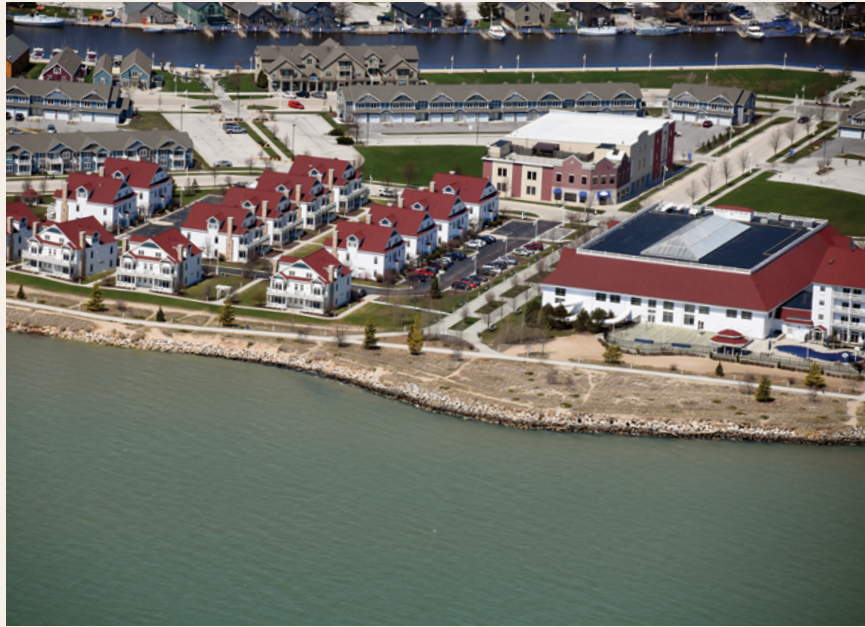
After Nourishment – High Lake Levels (2019) Beach has been inundated by high water levels. Sand that had buried the revetment has been eroded but the now-exposed revetment is preventing further erosion. Capt. Dennis Carr
