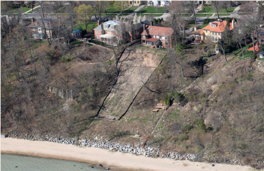
Before Oblique aerial image (2012) of the site before stabilization with a relatively unvegetated upper bluff slope, especially the particularly steep section just feet from the residence. USACE
