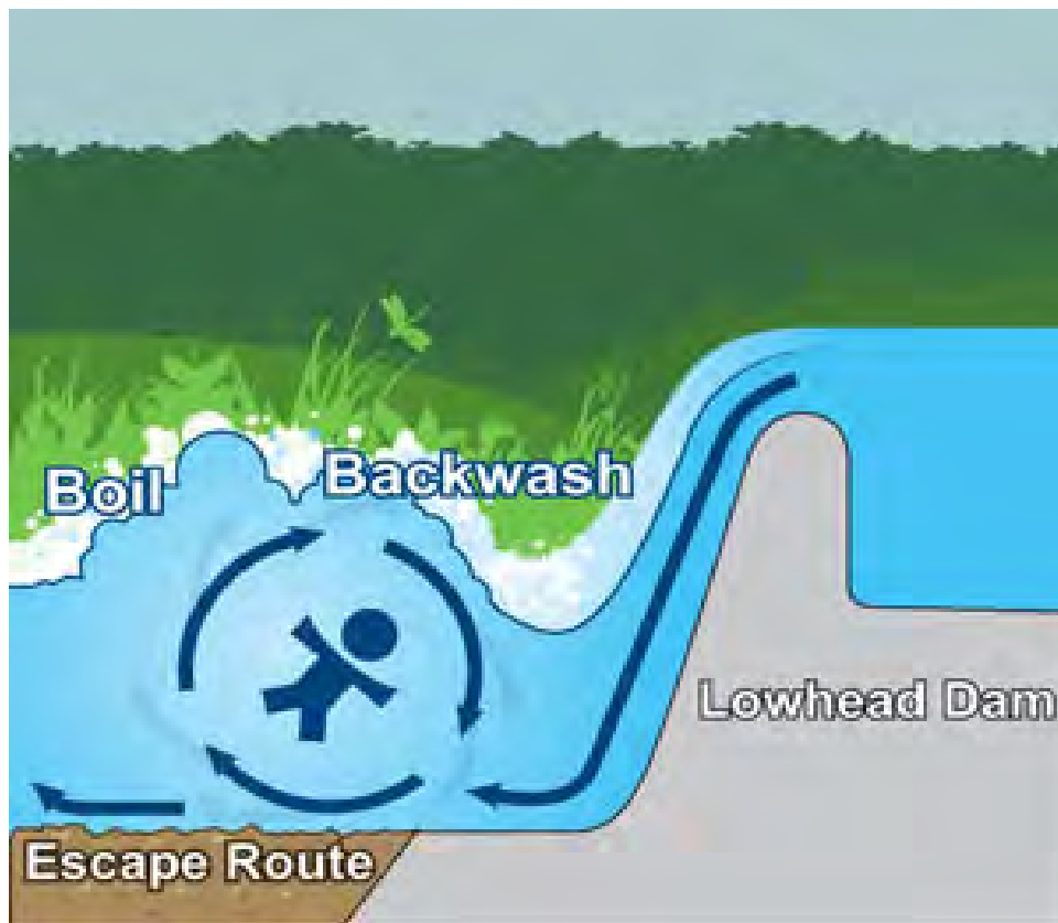
A significant safety problem with lowhead dams is created by the hydraulic conditions at the downstream base of the dam.
