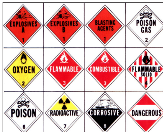
Figure 9.17. Hazardous materials warning placards.
