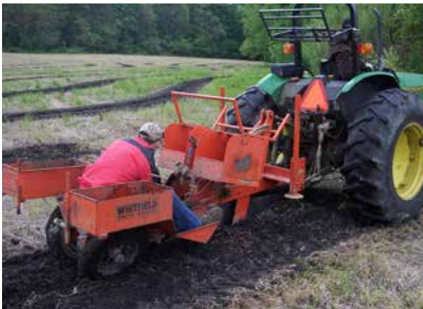
Figure 43. A tractor pulling a mechanized tree planter.
