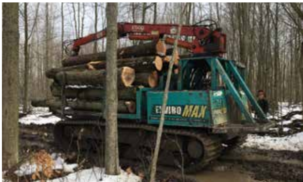
Figure 38. A tracked log forwarder designed to minimize impact to poorly drained soils.
