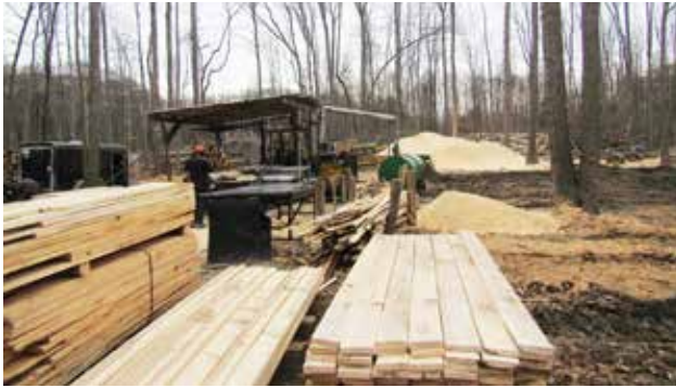
Figure 39. Portable sawmill in operation.
