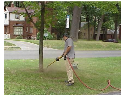
Air Spade ® uses high-pressure air to remove soil without damaging roots.
