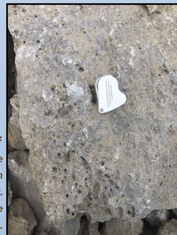
Figure 2. Example of vuggy porosity in the Lockport Dolomite from Genoa, Ohio quarry. Hand lens for scale (approx. 5 cm in length).
