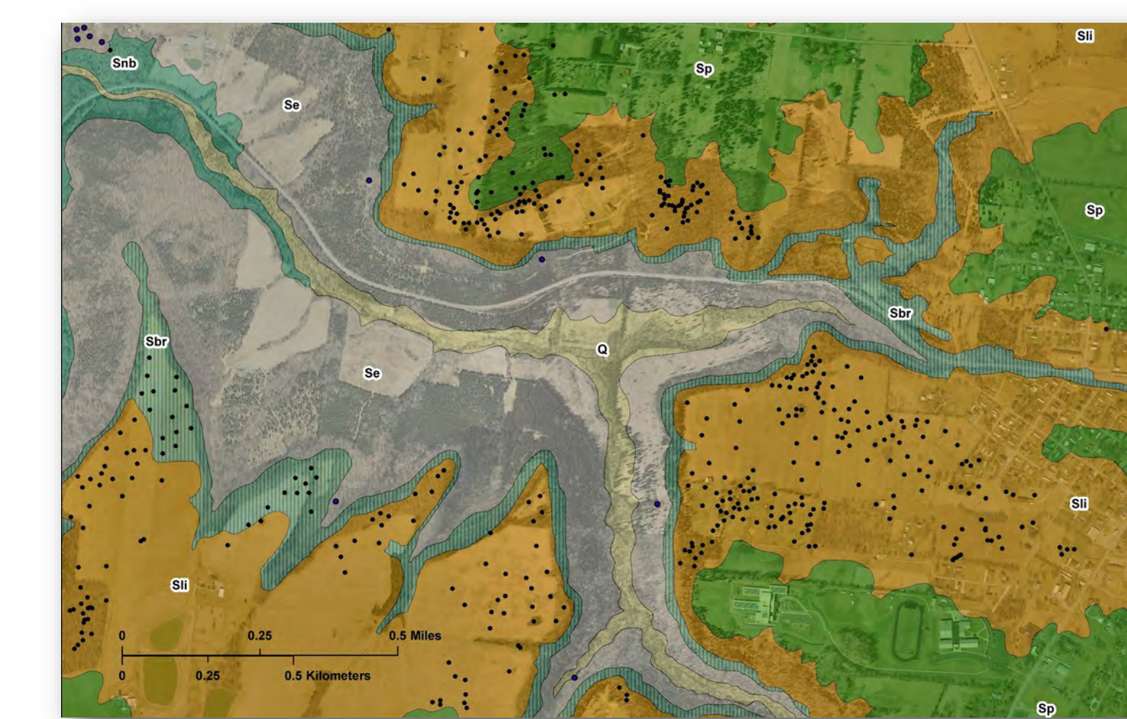
Figure 9. The majority of sinkholes form within the Lilley Formation (Sli, yellow). Note the large depression in the south east. Some sinkholes are forming stratigraphically above in the Peebles Formation (Sp, green), and some below in the Bisher Formation (Sbr, blue). See Figure 10.
