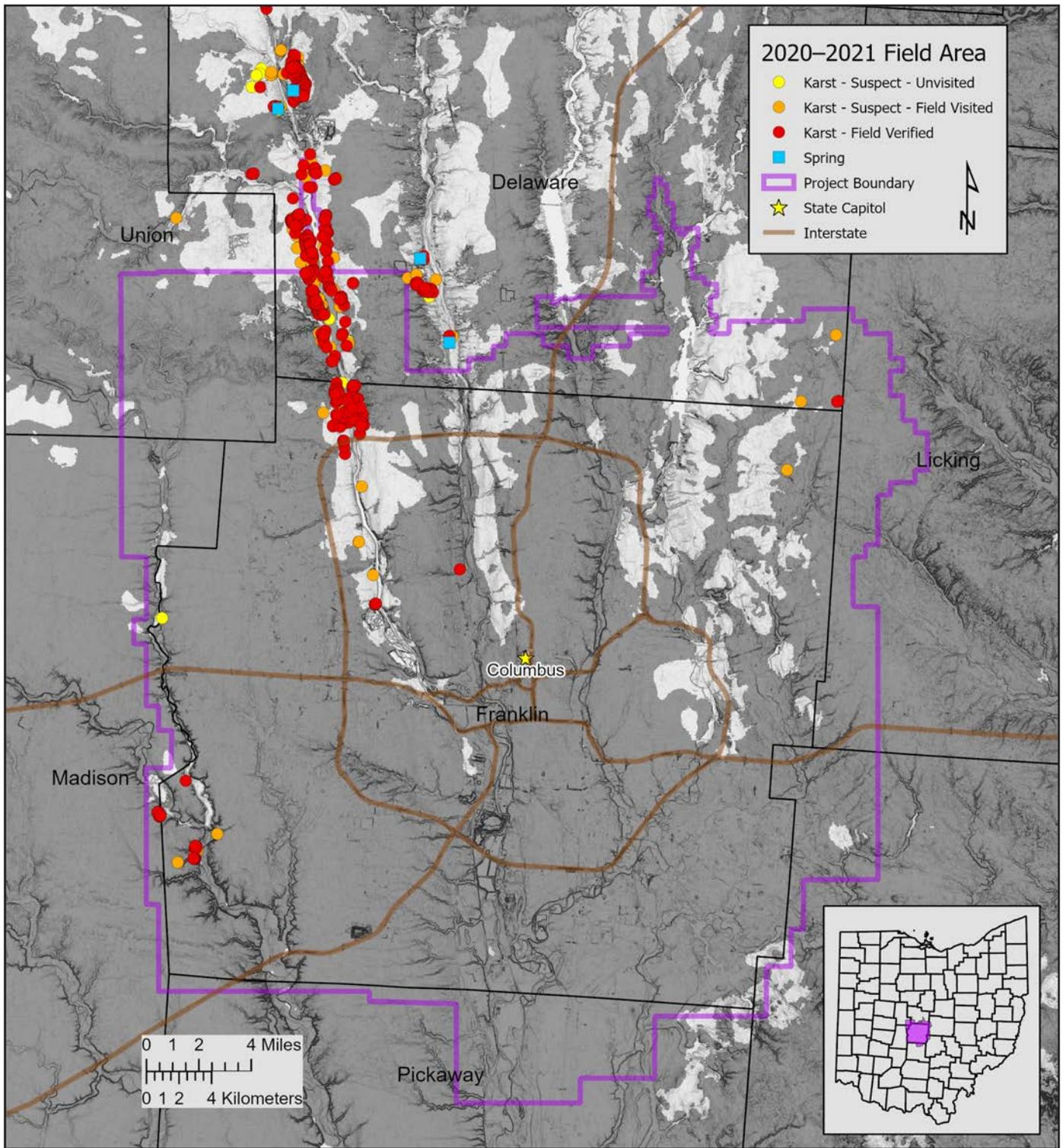
FIGURE 9. Map depicting the 2020-2021 study area (purple outline) in central Ohio where new 2015 LiDAR data was used. Dark gray areas (majority) are covered by more than 25 ft of glacial material at the surface and light gray areas are covered by less than 25 ft of glacial material at the surface. Note that the karst points are found almost exclusively in the light gray areas where the glacial material is thin.
