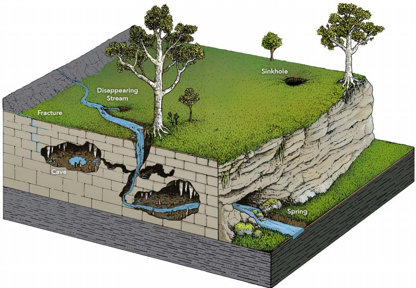
FIGURE 2. Block diagram showing the relationships between karst features. Illustration by Madison Perry.
