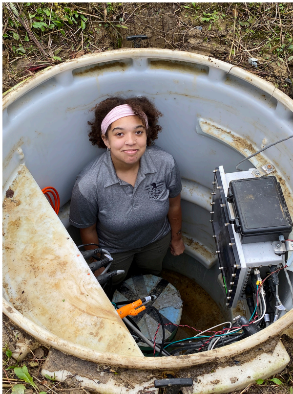
FIGURE A-9. ODNR intern assisting with field work maintenance of O53A in Harrison County, left, site overview on right. Seismometer is in tube at intern's feet.
