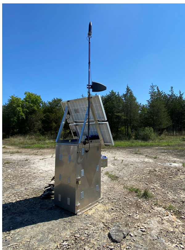
FIGURE A-2. Old style antennas and orientation on left was comprised of two small omni-directional antennas. The new style antennas consisting of a stronger omni-directional and directional antenna in their new orientation shown on the right.
