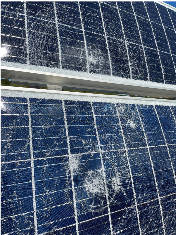
FIGURE A-7. Damaged solar panels at OhioSeis station KIOH (Kelleys Island, Ohio) were replaced in August of 2022.
