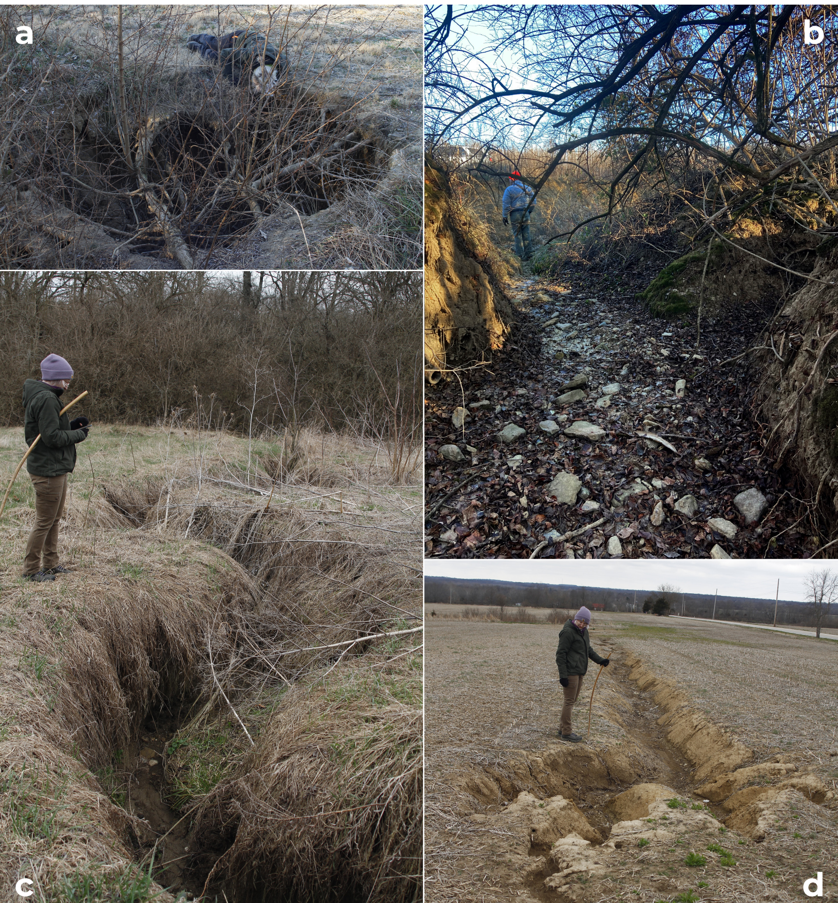
FIGURE 11. Four dramatic examples of erosion in farm fields in Butler County, Ohio, that are false positives identified by LiDAR and are unrelated to karst. The hole seen in Figure 11a was found to be flooded by failing drain tile. The elongated ditch seen in Figure 11b was determined to be a network of washed-out drain tiles in easily eroded silt along the edge of a farm field. The channel seen in Figure 11c was found to be a meandering stream cutting into farm pasture. The long erosional depression seen in Figure 11d was created by surface runoff.
