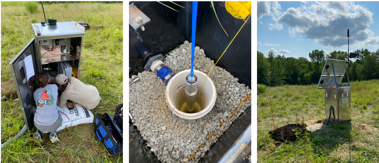
FIGURE A-4. Photos taken at OhioSeis station CROH at Carlisle Reservation in Lorain County, Ohio. Left: Intern and staff assembling power control system. Center: Using the downhole camera for aligning the seismometer at the bottom of the hole. Right: The operational station.
