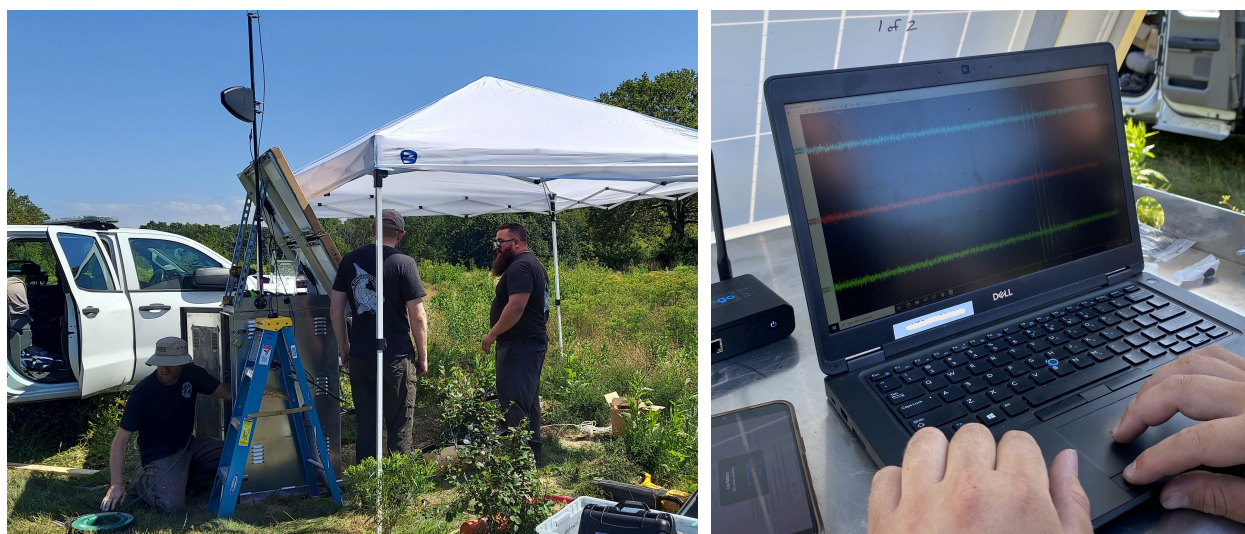
FIGURE A-3. Photos taken at OhioSeis station RBOH at Red Brook Metro Park in Ashtabula County, Ohio. Left: Installation of the site. Right: Checking seismic data produced at the newly installed station.
