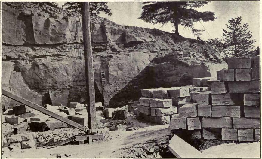
B.—Quarry in Mahoning sandstone at Corning, Perry County. The rock is used for bridges, foundations and viaducts. Photograph by D. D. Condit.
