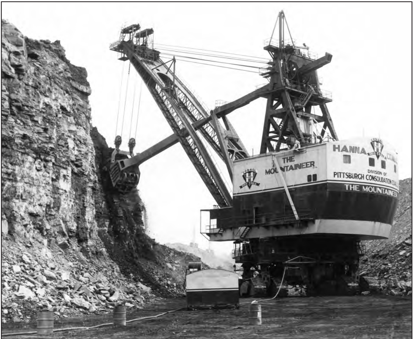
FIGURE 10.—The power shovel Mountaineer excavating overburden to expose an underlying seam of coal. This scene was typical for the Mountaineer , which was operated by the Hanna Coal Company, Division of Pittsburgh Consolidation Coal Company, in surface mines of southern Harrison and northern Belmont Counties from 1956 to 1979. The Hanna Coal Company was formed in 1900 as Wheeling and Lake Erie Coal Company. In 1931 the name was formally changed to Hanna Coal Company. During World War II, the Hanna Coal Company was informally referred to as the United States Coal Company. In June 1946, Hanna Coal Company became a Division of Pittsburgh Consolidation Coal Company. In 1958, the corporate name was shortened to Consolidation Coal Company, more commonly known as Consol. Circa 1970's. Photo courtesy of Dale Davis.
