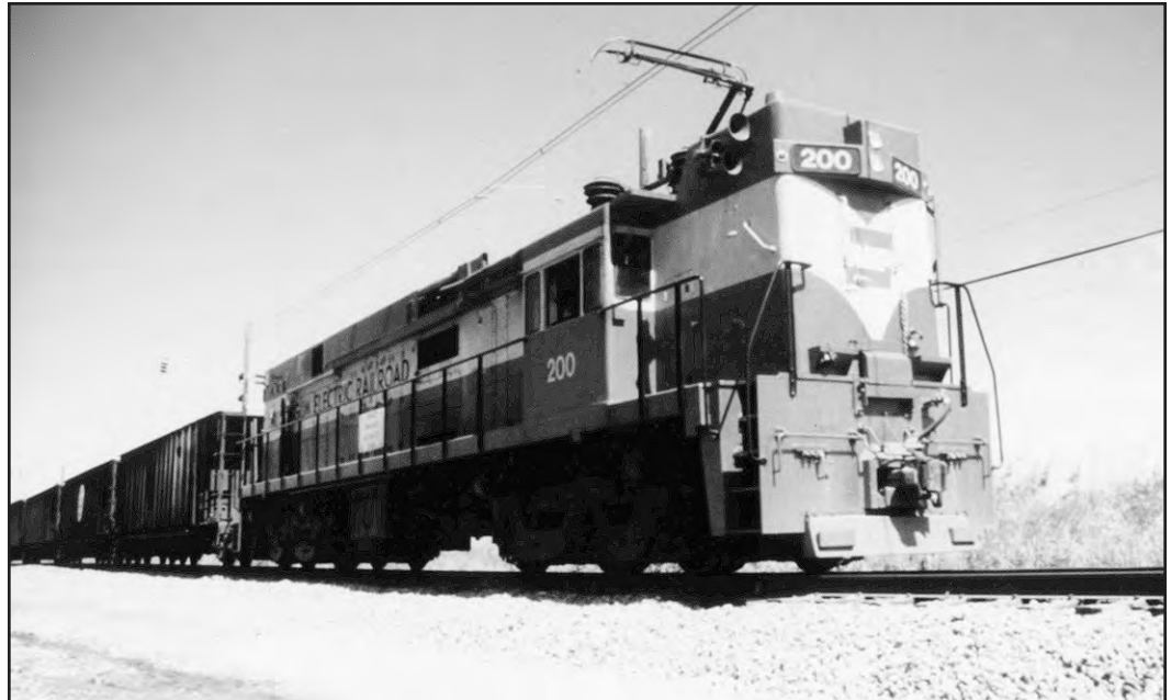
FIGURE 13.—Central Ohio Coal Company's Muskingum Electric Railroad, the first totally electric, fully automated railroad in North America, moves coal from the mine's loading area to its coal preparation plant 15 miles away. The Meigs Creek (No. 9) coal is mined from Central Ohio Coal Company's Muskingum mine (Ne-41) and used at Ohio Power Company's Muskingum River electric-generating station. Circa 1988. Photo courtesy of American Electric Power Service Corporation. (For other photos of this mine see figs. 11 and 200.)
