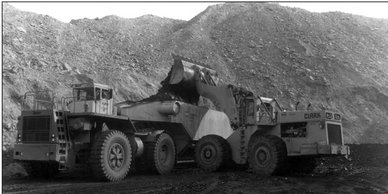
FIGURE 28.—Hydraulically actuated front-end loader loading Meigs Creek (No. 9) coal into a 160-ton coal hauler at the Central Ohio Coal Company Muskingum mine (Ne-41), located in Muskingum, Noble, and Morgan Counties. Circa 1988. Ohio Division of Geological Survey file photo.
