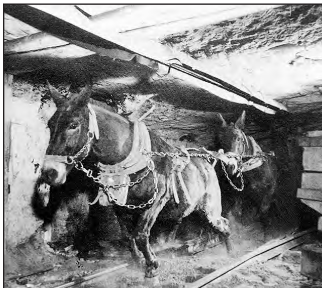
FIGURE 95.—Mules straining against their harnesses to pull a loaded coal car. Date and location unknown. Photo courtesy of Forrest Walton.
