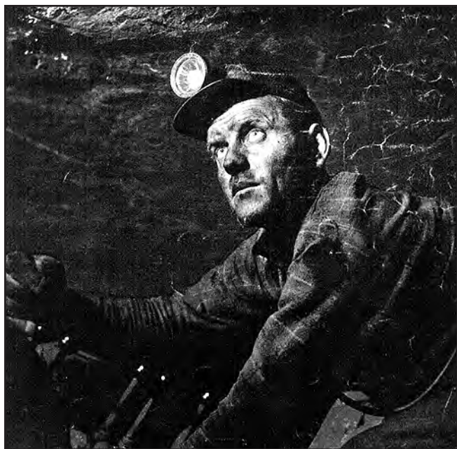
FIGURE 100.—Dick Beamer, age 38, wears a battery-powered electric miner's lamp as he operates a coal-cutting machine in the Midvale No. 7 mine (Ts-389), about 2 miles east of Midvale, in Union Township, Tuscarawas County. This slope mine was operated by the Columbia Southern Chemical Corporation (formerly by the Midvale Coal Company, Inc.) and produced Middle Kittanning (No. 6) coal until it was abandoned in 1971. Photo by NEWSWEEK-O.C. Sweet, cover ©1947, Newsweek, Inc. All rights reserved. Reprinted by permission.
