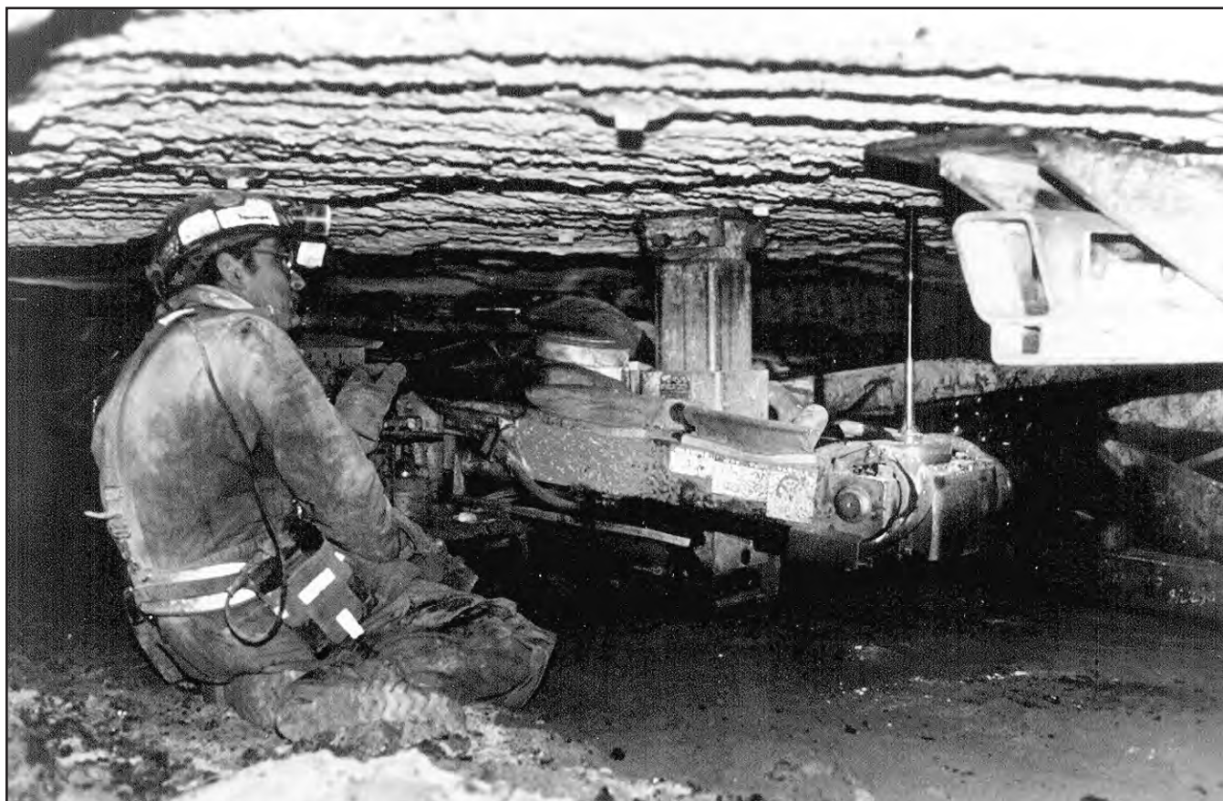
FIGURE 114.—A coal miner operating a Fletcher II roof bolter in the Sterling mine (Jfn-823), a drift mine operated by the Sterling Mining Corporation in Brush Creek Township, Jefferson County. Note the confined height in which this miner is working. Photo taken in 1993. Photo courtesy of Tim Miller. (For other photos of this mine see figs. 87 and 88.)
