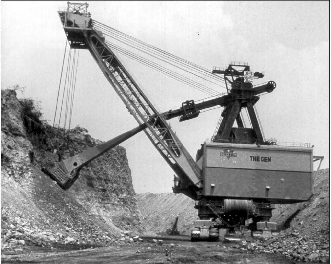
FIGURE 26.—The GEM , built by Bucyrus-Erie, stood taller than a 12-story building and had a 105-cubic-yard bucket capacity. This electric-powered shovel was operated by the Consolidation Coal Company in the Mahoning Valley No. 33 surface mine (Hn-700) near Cadiz in Athens and Short Creek Townships, Harrison County. Circa late 1970's. Ohio Division of Geological Survey file photo.
