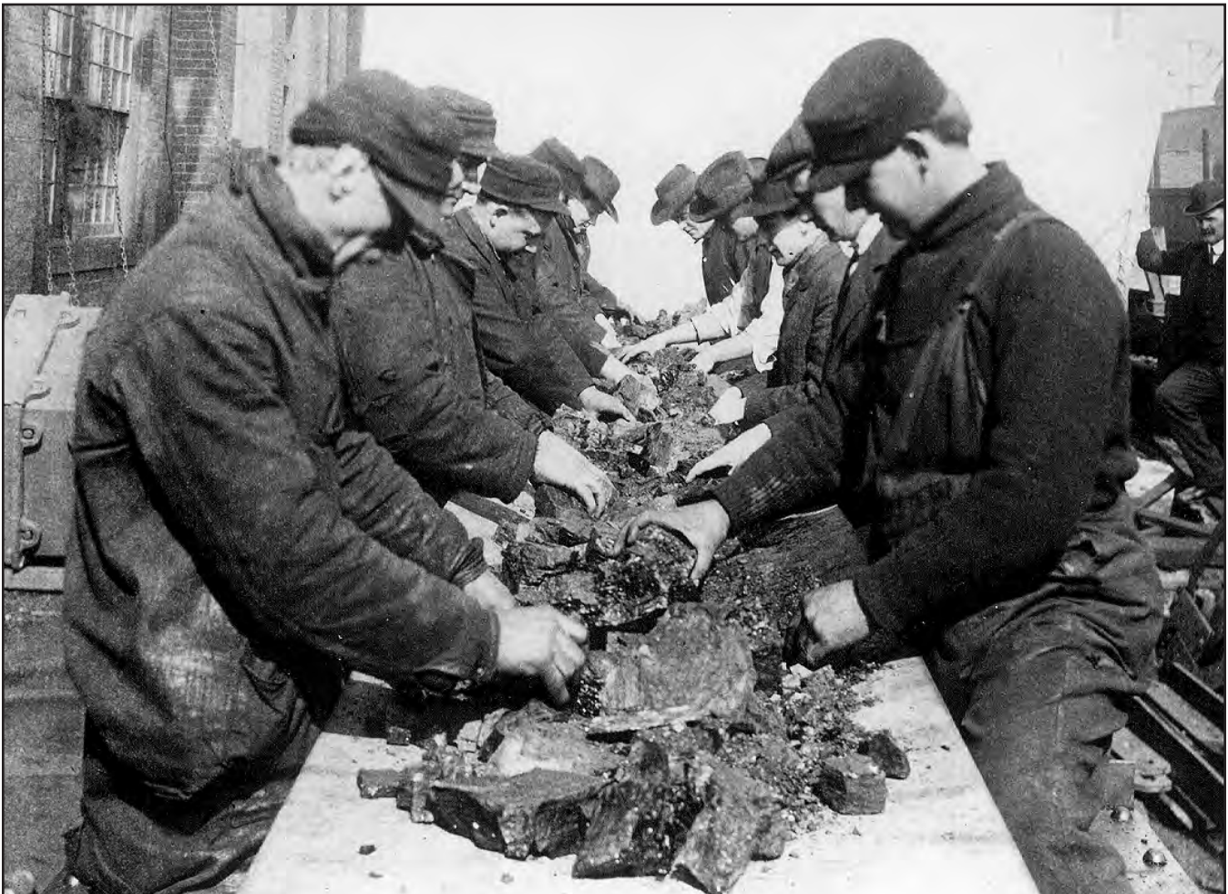
FIGURE 218.—Early coal cleaning involved separation by hand of the waste material from the coal as the coal passed by the "pickers" on a conveyor. Circa early 1900's. Location unknown. Photo courtesy of Ohio Historical Society, from the Jeffrey Mining Equipment Company collection.
