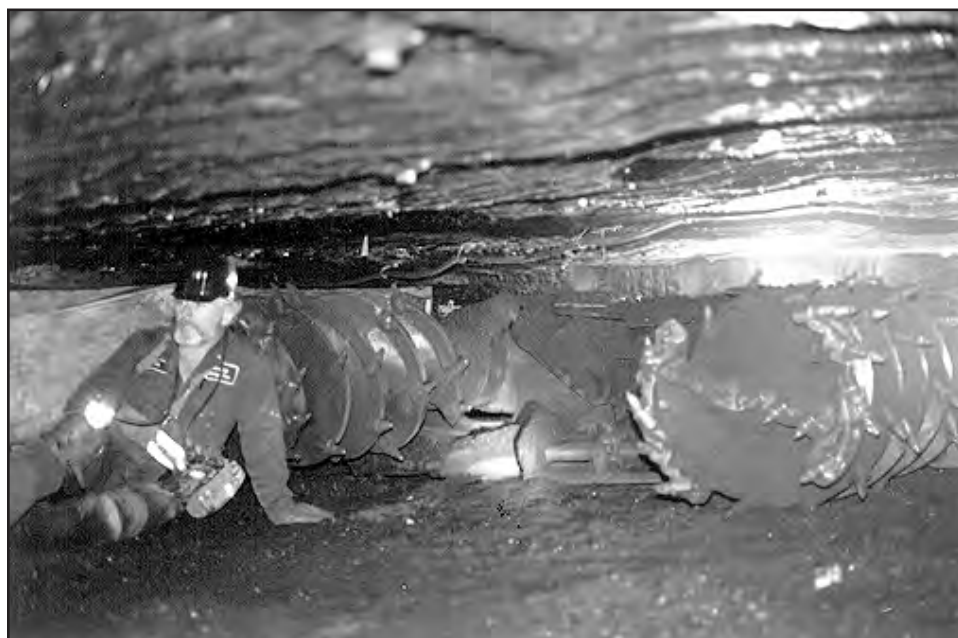
FIGURE 87.—Top photo, head-on view of a Fairchild 410 auger-style continuous miner making a cross-cut entry through a pillar of coal in the Sterling mine (Jfn-823) in Brush Creek Township, Jefferson County. Bottom photo, the same continuous miner at idle. This continuous miner uses two rotating cylinders (augers), 32 inches in diameter and studded with tungsten carbide bits, extended on arms which swing horizontally side to side and raise and lower vertically. When this continuous miner is in operation, water is continuously sprayed to retard the generation of coal dust. The coal seam in this mine is the Mahoning (No. 7A), and mine height averages 35 inches. Photo taken in 1992. Photo courtesy of Tim Miller. (For other photos of this mine see figs. 88 and 114.)
