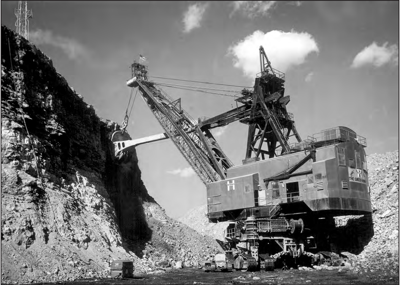
FIGURE 25.—The Green Hornet , a 50-cubic-yard capacity, electric-powered Marion 5561 shovel. This shovel was operated by the Hanna Coal Company at the Georgetown No. 12 surface mine in Athens and Short Creek Townships, Harrison County. Circa 1950's. Ohio Division of Geological Survey file photo.
