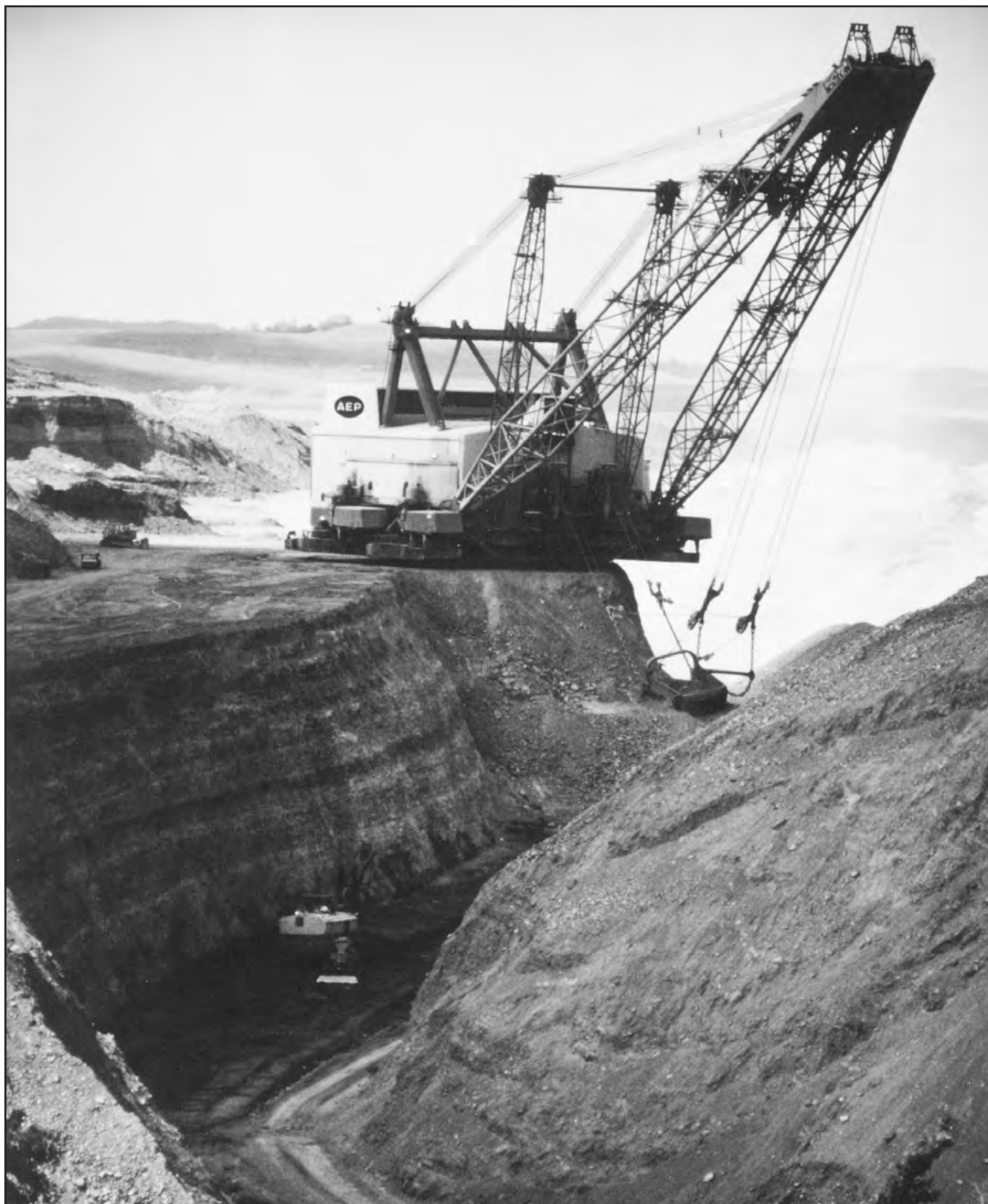
FIGURE 11.—The Big Muskie , built by Bucyrus-Erie, is the world's largest walking dragline machine. This dragline has a 220-cubic-yard capacity bucket and was operated from 1969 to 1991 by the Central Ohio Coal Company at the Muskingum mine (Ne-41), located near Coal Hill, Meigs Township, Muskingum County. The Big Muskie has been idle since 1991. Photo taken by Doug Crowell in 1984. (For other photos of this mine see figs. 13 and 200.)
