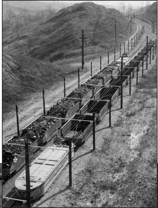
FIGURE 36.—A loaded “trip” or train of mine cars, led by a 20-ton haulage locomotive, leaving the Hanna Coal Company Piney Fork No. 1 mine (Jfn-243), passing a string of empties preparing to enter the mine. Circa 1955. Photo courtesy of Hanna Coal Company. (For other photos of this mine see figs. 74, 101, 116, 121, 159.)
