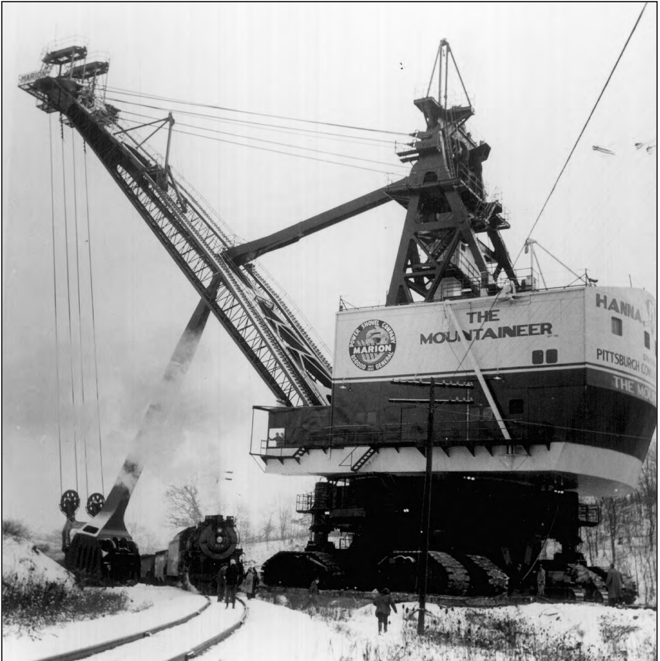
FIGURE 24.—The Mountaineer , an electric-powered shovel built by the Marion Power Shovel Company and heralded as the world's largest shovel in 1956. The Mountaineer is seen here alongside one of the last coal-fired steam locomotives operating commercially in Ohio's coal fields. Circa 1956. Photo courtesy of Ohio Historical Society.
