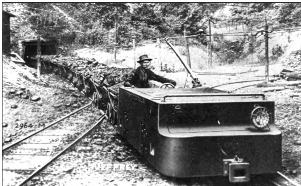
FIGURE 34.—Ten-ton electric locomotive manufactured by Jeffrey Mining Equipment Company towing a shuttle train loaded with coal from the Alma mine (Vn-18) operated by the Alma Cement Company. This drift mine, located near Oreton, Vinton Township, Vinton County, produced both Clarion (No. 4A) coal and Vanport limestone. It was abandoned in 1909. The mine was reopened by the Manhattan Coal Company and finally abandoned in 1924. Circa 1908. Photo from State Inspector of Mines Report (1909, p. 100).
