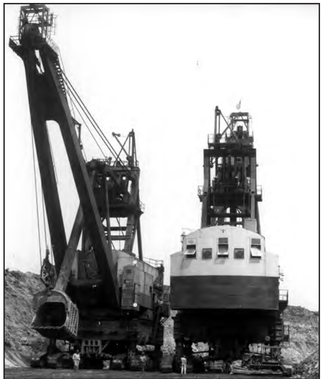
FIGURE 23.—Side-by-side view of Hanna Coal Company's A (right) and B (left) shovels in a surface mine near Georgetown. Both shovels are 35-cubic-yard capacity, Marion 5561 electric-powered shovels. Circa 1947. Photo courtesy of Dale Davis. (For another photo of this mine see fig. 50.)
