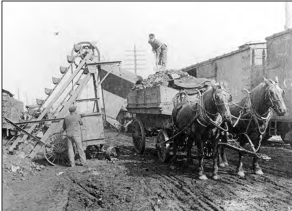
FIGURE 197.—Bucket-conveyor wagon loader loading a horse-drawn wagon at the railyards in Toledo. The coal was shipped by the Big Four Coal Company. Circa early 1900's. Photo courtesy of Ohio Historical Society, from the Jeffrey Mining Equipment Company collection.
