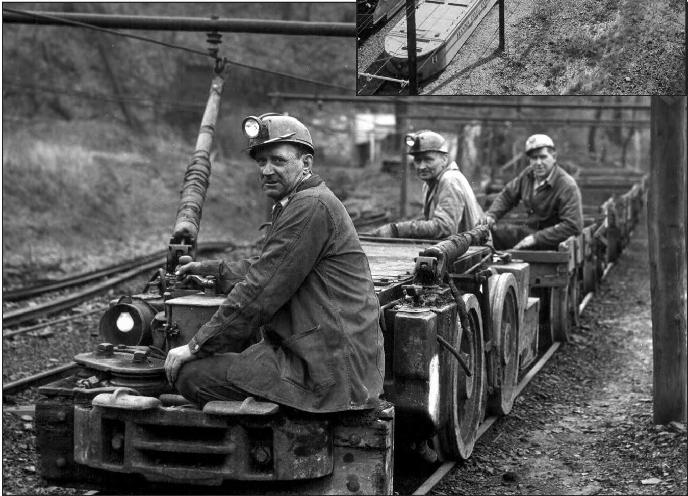
FIGURE 37.—Coal miners riding an electric shuttle train en route to an eastern Ohio mine. Shuttle trains carrying miners to and from the mine are commonly referred to as man trips. Date and location unknown. Photo courtesy of Ohio Department of Industrial Relations, Division of Mines.
