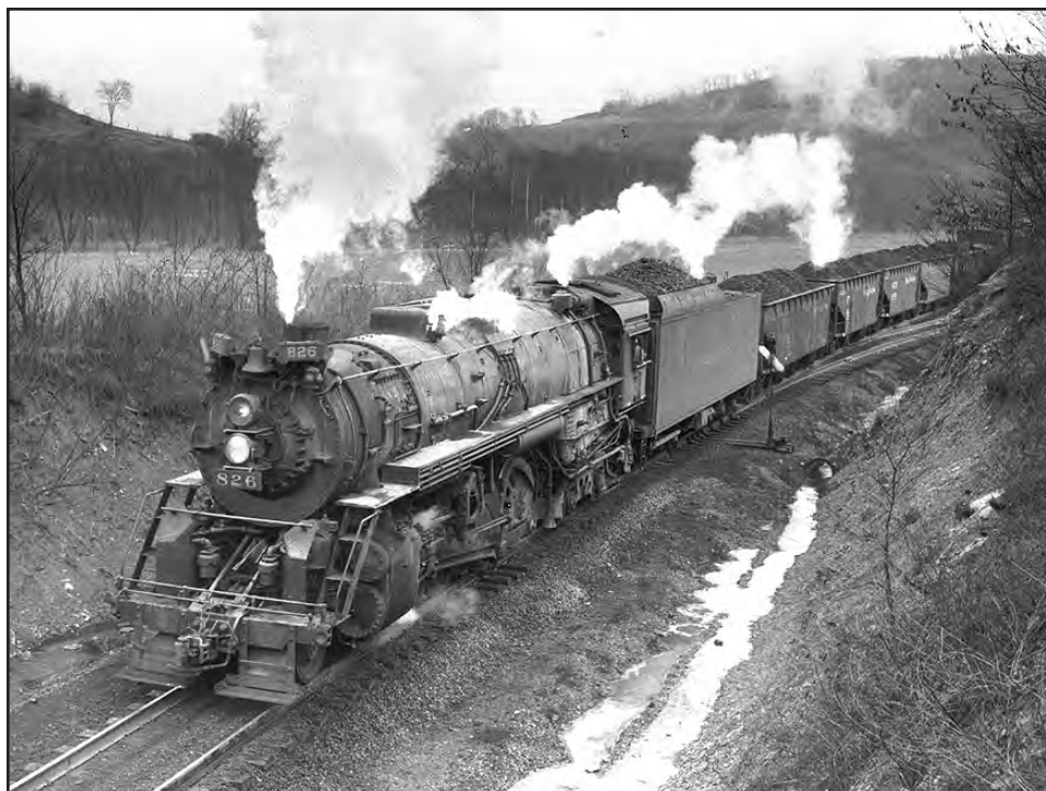
FIGURE 187.—Nickel Plate Railroad 2-8-4 #826 (nee W & LE #6426) about to cut away from the caboose and back onto pick-up tracks to fill out the train's tonnage with coal from the Saginaw mine (Bt-643) before heading to Adena and Pine Valley in Jefferson County. The Saginaw mine, a slope mine in the Pittsburgh (No. 8) coal located just southwest of St. Clairsville, in Richland Township, Belmont County, was operated by the Saginaw Mining Company and ceased operations in December 1992. Circa 1956. Photo and information on engine courtesy of J. J. Young, Jr.
