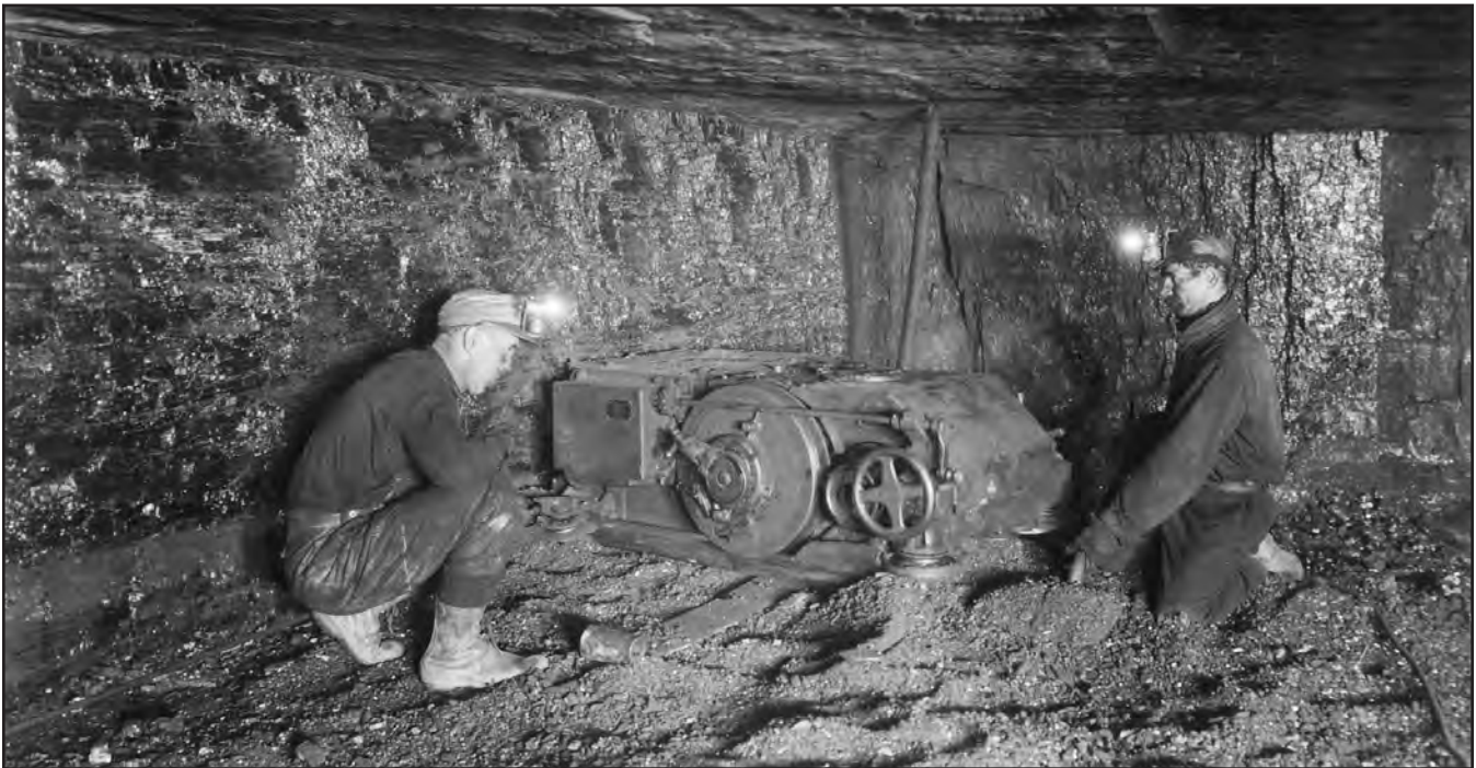
FIGURE 33.—Two miners undercutting a seam of coal in an eastern Ohio coal mine using a coal-cutting machine built by Jeffrey Mining Equipment Company. Note the low ceiling and the carbide lamps and cloth hats worn by the miners. Date and location unknown. Ohio Division of Geological Survey file photo.
