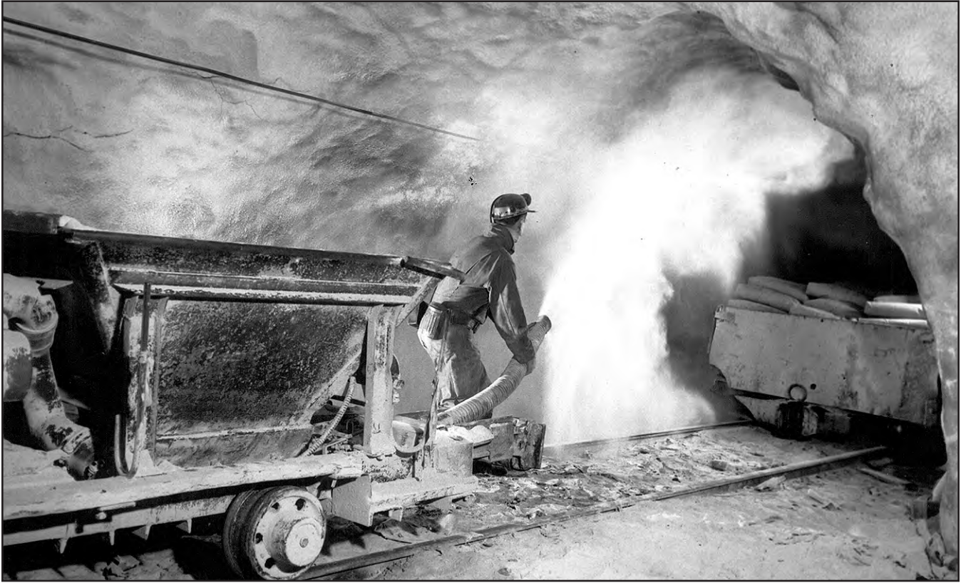
FIGURE 115.—A powerful blower sprays the underground roof and walls [of a Hanna Coal Company mine in eastern Ohio] with "rock dust"-lime rock ground as fine as talcum powder. This dilutes the coal dust, neutralizes its explosive qualities, and safeguards against explosions (Bituminous Coal Institute in Newsweek, 1947, v. 30, p. 9). Circa 1950. Ohio Division of Geological Survey file photo.
