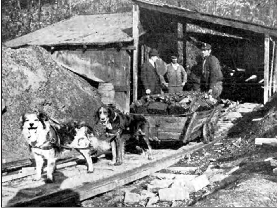
FIGURE 96.—Dogs commonly were used to pull mine cars at coal mines primarily in Muskingum County during the 19th and early 20th centuries. Photo from The Coal Trade Bulletin (1922, v. 47, no. 9, p. 352).
