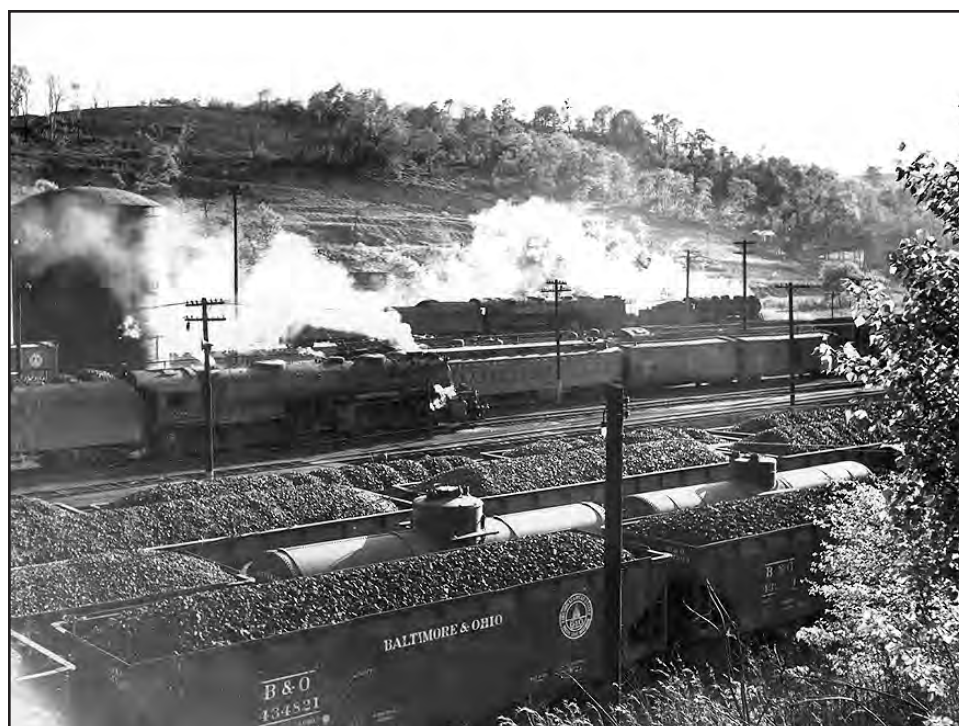
FIGURE 188.—In the B & O yards at Holloway (Belmont County) an L-2 0-8-0 takes an EM-1 2-8-8-4 (background) to be loaded with coal and water. A sister EM-1, #7629 (center), awaits a call to take coal to the port of Lorain. Photo taken in October 1953. Photo and information courtesy of J. J. Young, Jr.
