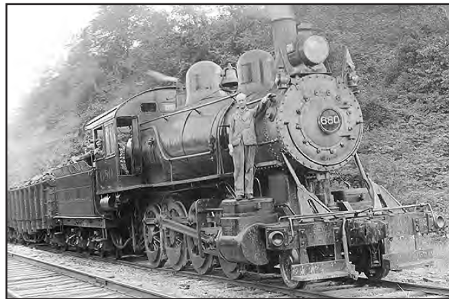
FIGURE 193.—W & LE 2-8-0 #680 hauling a load of Pittsburgh (No. 8) coal from the Hanna Coal Company Willow Grove No. 10 mine (Bt-163). Circa 1917. Photo courtesy of Charles "Bud" Fry. (For other photos of this mine see figs. 35, 79, 82, 93, 110, 117, 119, 120, 123, 140-142, 153, 154.)
