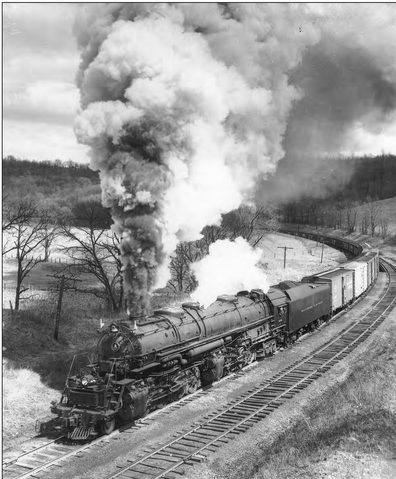
FIGURE 184.—B & O EM-1 2-8-8-4 #676 hauling a Holloway Humper through Bannock (Belmont County) on a brisk November afternoon in 1957. Hauling 97 cars carrying 8,700 tons of coal, the EM-1 pulls mightily to get the train to the summit at Flushing (Belmont County). Holloway Humper is a term applied to trains bringing coal out of the Ohio Valley over the summit at Flushing to be assembled into longer trains at the railyards in nearby Holloway for shipment to Lake Erie ports. Photo and information on engine courtesy of J. J. Young, Jr.
