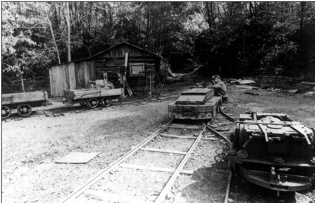
FIGURE 38.—Converging tracks lead through the trees in the background to Ray Stahl's one-man coal mine. Stahl built most of his equipment, including the locomotive he's driving. The machine on the right, mounted on rails, is a coal cutter which Stahl used to mine about 4 tons of coal per day. The mine cars on the left each hold about 1,700 pounds of coal, which Stahl would load by hand. Photo by Fred Shannon, from the Columbus Dispatch Sunday Magazine, January 28, 1979, p. 9. Reprinted with permission. (See also cover photo.)
