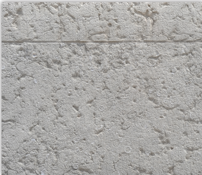
Columbus Limestone of the Ohio Statehouse in Columbus, Franklin County. Numerous fossils can be found in the exterior walls, stairs, and columns of the statehouse.
