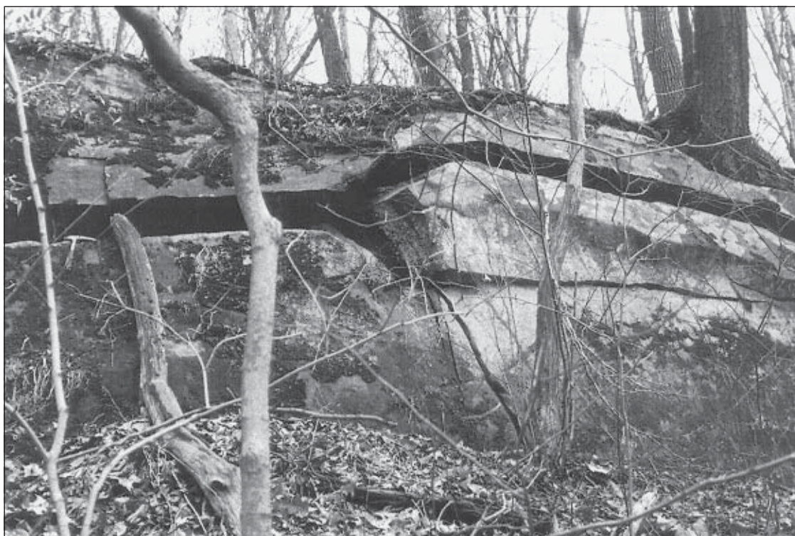
FIGURE 17.—Bedding separation in the Lower Freeport sandstone overlying the Majestic Mine. Rock hammer at left center for scale.
