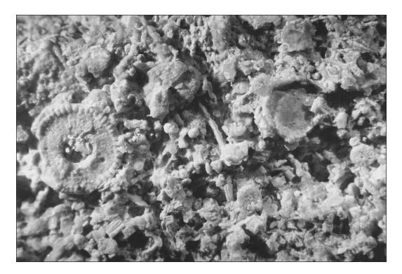
FIGURE 63.—Closeup view of Salem Limestone, also known as *Indiana limestone* (from Hannibal and Schmidt, 1992, p. 6). The wheelshaped fossil to the left is a segment of the stem of a sea lily. It is about 3 mm in diameter.
