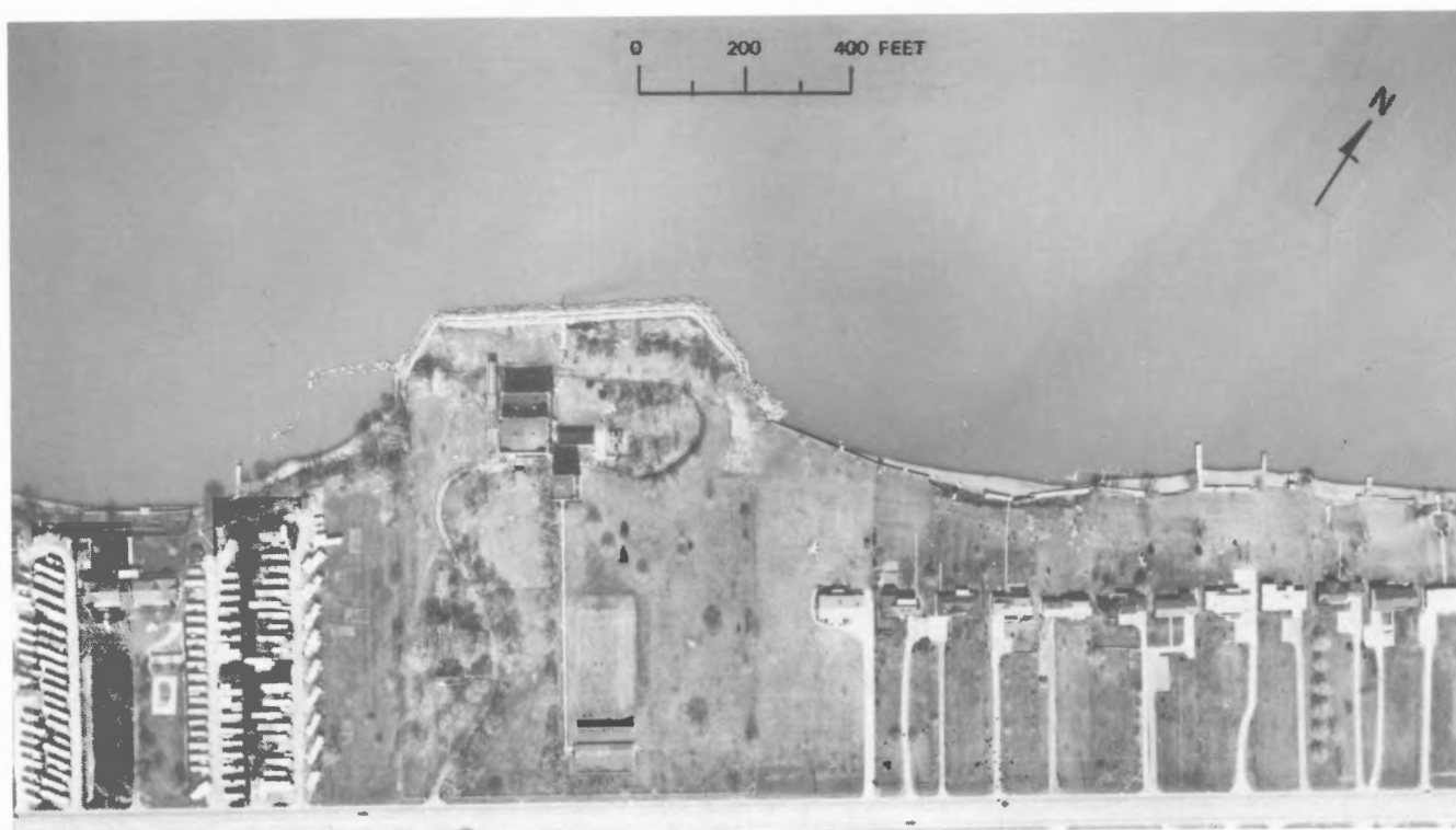
FIGURE 16.—STOP 13, Elyria waterworks. Rubble-mound seawall fronting the waterworks complex.
