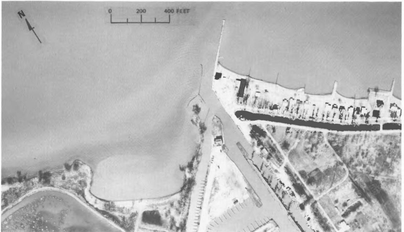
FIGURE 4.—STOP 2, Reno Beach, Lakemont Landing. A good example of a well-protected updrift (southeast) shoreline and an unprotected downdrift (northwest) shoreline.
