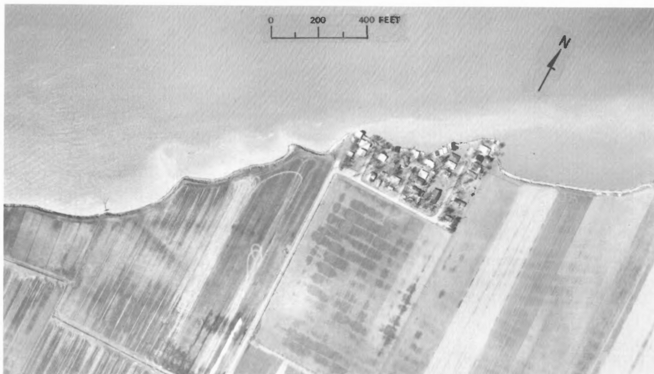
FIGURE 10.—STOP 8, Crystal Rock. Unprotected clay banks; waves breaking on nearly demolished manmade structure just offshore.
