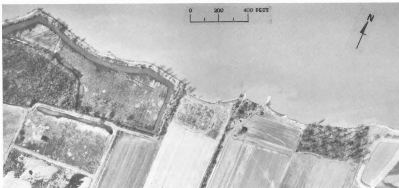
FIGURE 11.—STOP 9, Willow Point. Quarry-run stone dike adjacent to unprotected embayed shoreline.
