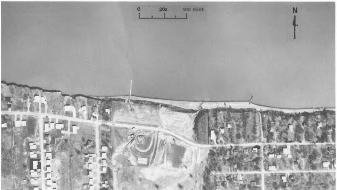
FIGURE 15.—STOP 12, Vermilion-on-the-Lake. Vertical shale bluff west of the groin and less resistant till bluff east of the groin.
