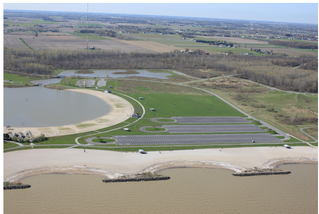
FIGURE 30. Aerial view of the sand beach at Maumee Bay State Park, Lucas County, Ohio, protected by offshore breakwaters. Image provided by the U.S. Army Corps of Engineers.
