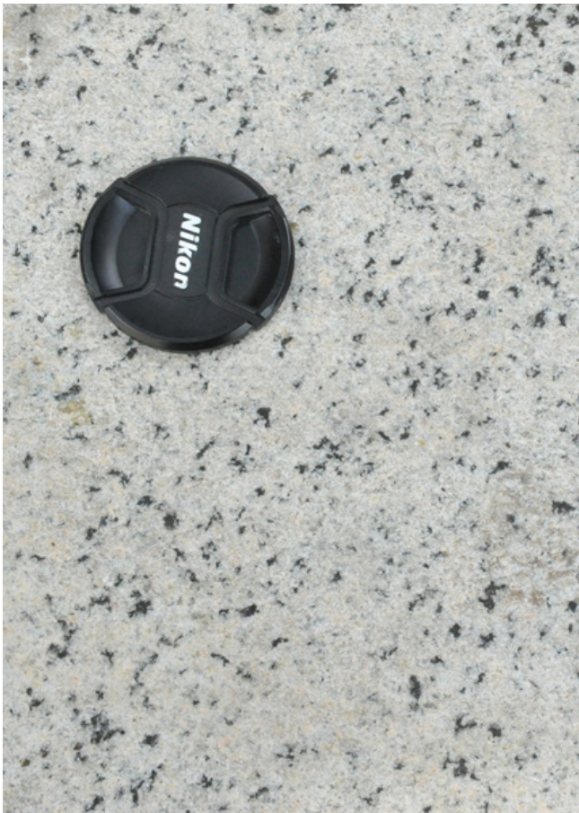
FIGURE 61. Close-up photograph of granite in Perry's Victory and International Peace Memorial on South Bass Island in Lake Erie. Lens cap for scale.
