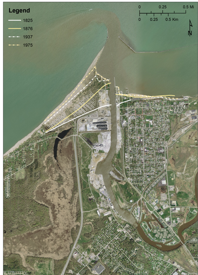
FIGURE 81. Historical shorelines superimposed on a 2011 aerial photograph of Headlands Beach and the mouth of the Grand River, Fairport Harbor, Ohio. Mentor Marsh is south of Headlands Beach. After Guy and Moore (2010, fig. 24).
