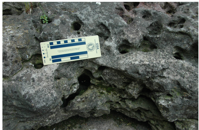
FIGURE 50. Honeycomb weathering in Columbus Limestone near base of Marblehead Lighthouse, Ottawa County, Ohio.
