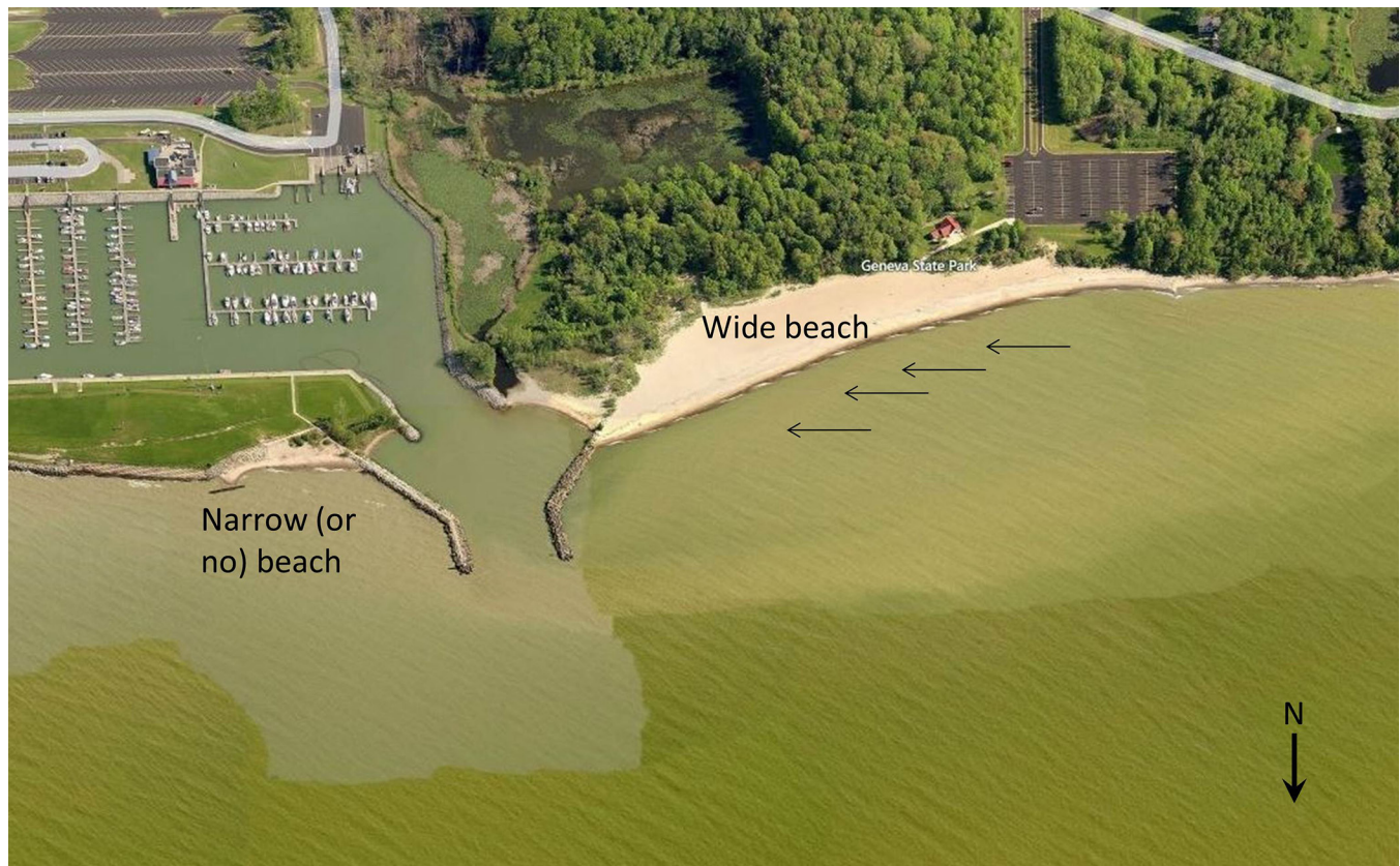
FIGURE 87. Low-angle aerial view of the beach and marina entrance channel at Geneva State Park, Ashtabula County, Ohio. Arrows show the net direction of longshore current, which is from west to east. Most sand is trapped at the western jetty and does not continue eastward.
