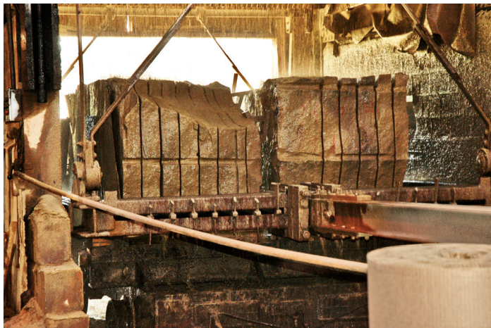
Gang saw being used to cut a block of Massillon sandstone into slabs at The Briar Hill Stone Company plant located in Glenmont, Ohio. Average sized blocks weigh approximately 10 tons.
