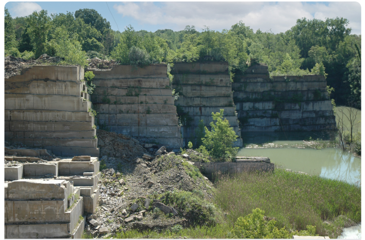
Figure 1. The Cleveland Quarries Birmingham quarry where two distinct colors of Berea Sandstone, known as “Birmingham Buff” and “Amherst Gray,” are found.
