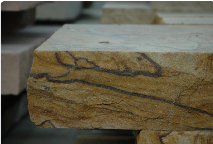
Figure 2. Massillon sandstone slab variety referred to as “copper variegated” at The Briar Hill Stone Company in Glenmont, Ohio. Iron banding gives it a signature look that is quite popular with customers.
