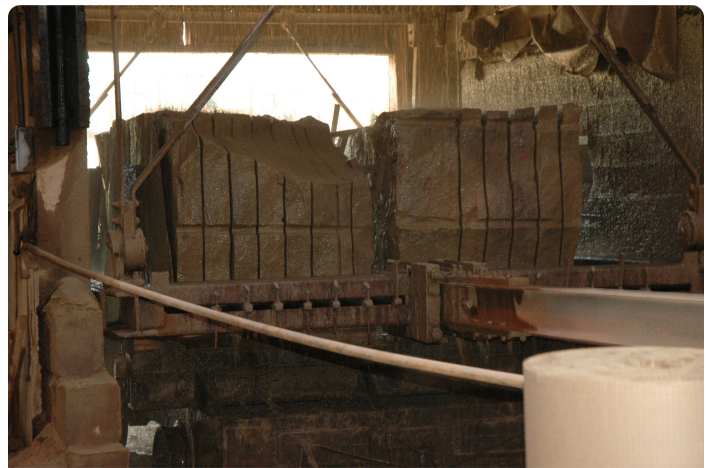
Figure 3. Gang saw being used to cut a block of Massillon sandstone into slabs at The Briar Hill Stone Company plant in Glenmont, Ohio. Average-sized blocks weigh approximately 10 tons.
