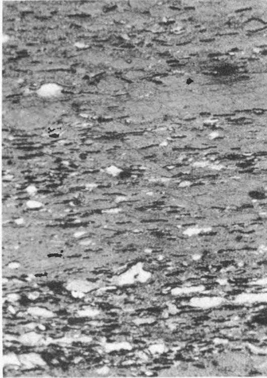
Fig. 16 - Bands of clarain with 7 per cent (top), 12 per cent (center), and 27 per cent (bottom) of spore exines as determined by dot-count. Pittsburgh (No. 8) bed coal, block 2, column 604. (From reference 1: Cady and Smith, 1955, p. 26, fig. 5.)
