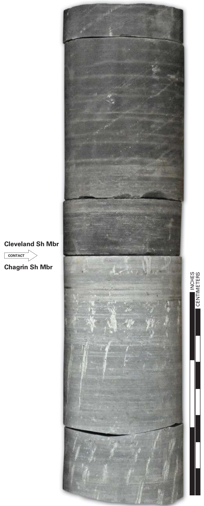
Black, organic-rich shale of the Cleveland Shale Mbr in contact with the gray shale of the Chagrin Shale Mbr
