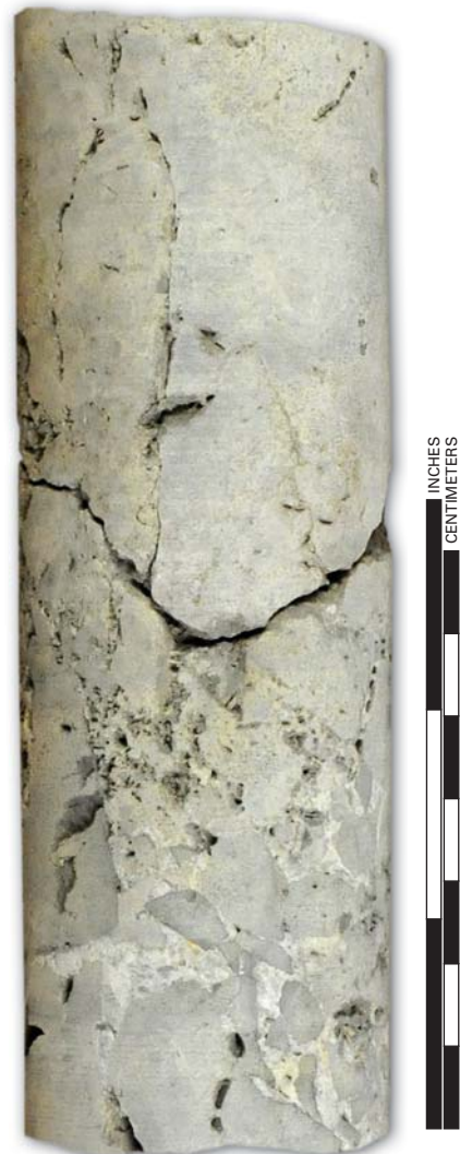
Fractured, angular, microcrystalline dolomite cemented with white calcite cement
