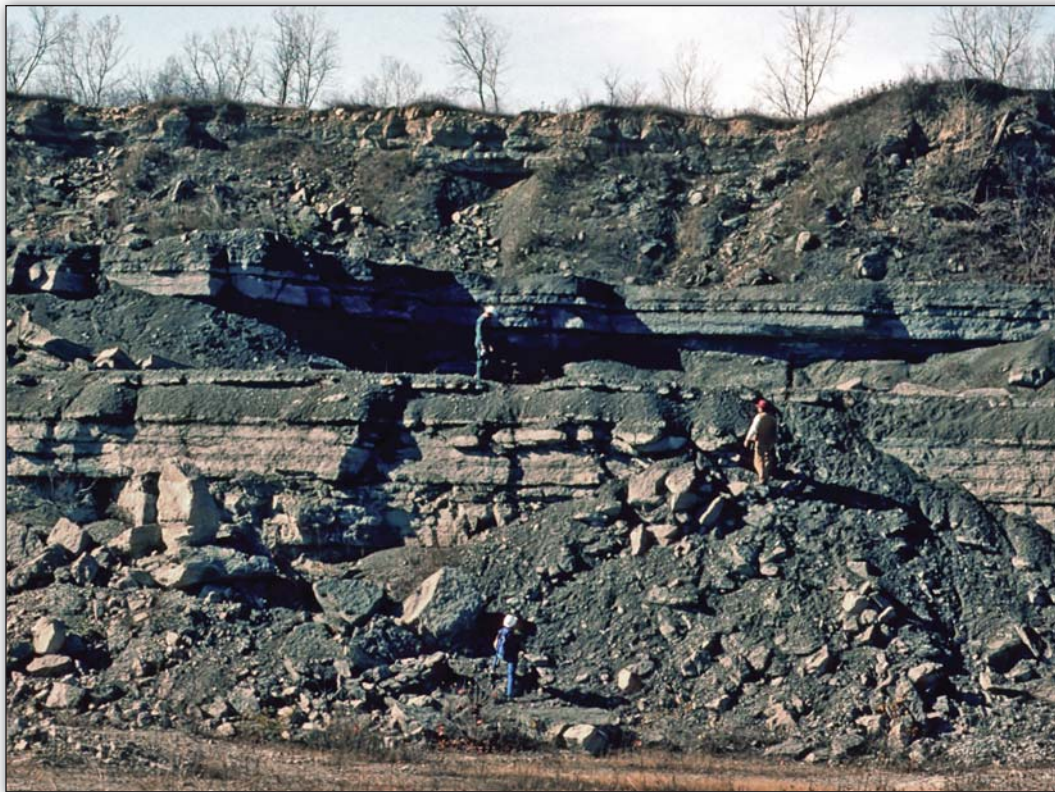
The Silica Formation of the Traverse Group characterized by planar bedded, fossiliferous, argillaceous limestone and calcareous, fossiliferous shale exposed by quarrying in the Medusa South Quarry of France Stone Company.
