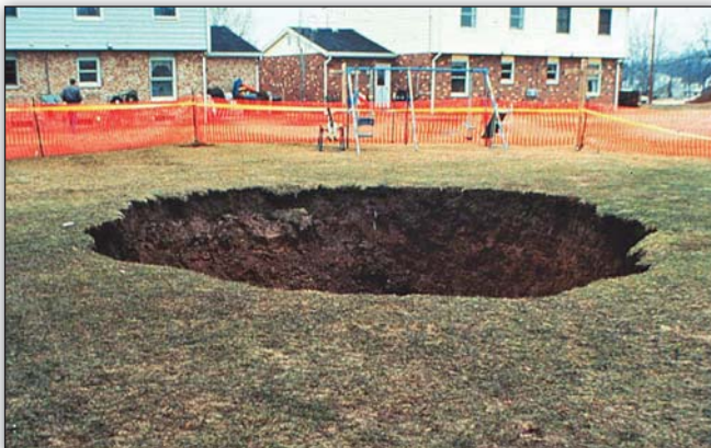
Mine subsidence pit measuring 35 ft across and 25 ft deep has opened in a residential area in North Canton, Stark County. These pits occur as the overlying strata collapses into the mined voids of abandoned or active underground mines. Mine subsidence is a major geologic hazard in areas with underground mining. See the Survey website, OhioGeology.com , for more information.
