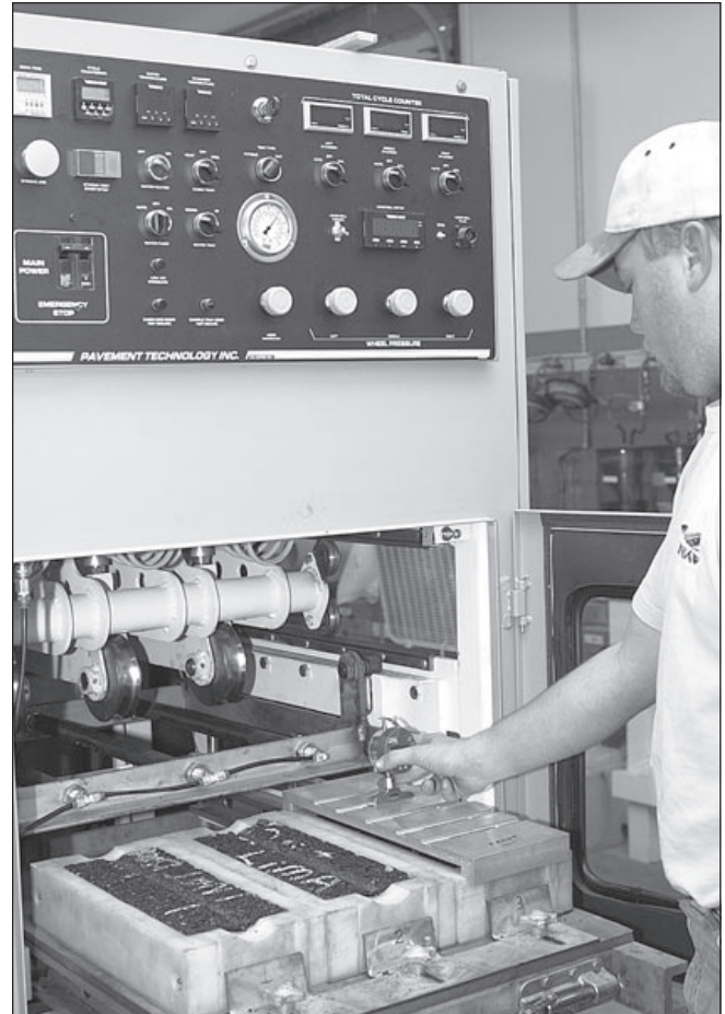
The asphalt pavement analyzer enables the contractor to estimate rutting susceptibility. Pictured here is lab technician Darrel Cooperrider at the quality control laboratory of The Shelly Company in Perry County. Photo by Michael D. Williams, Ohio Department of Natural Resources.
