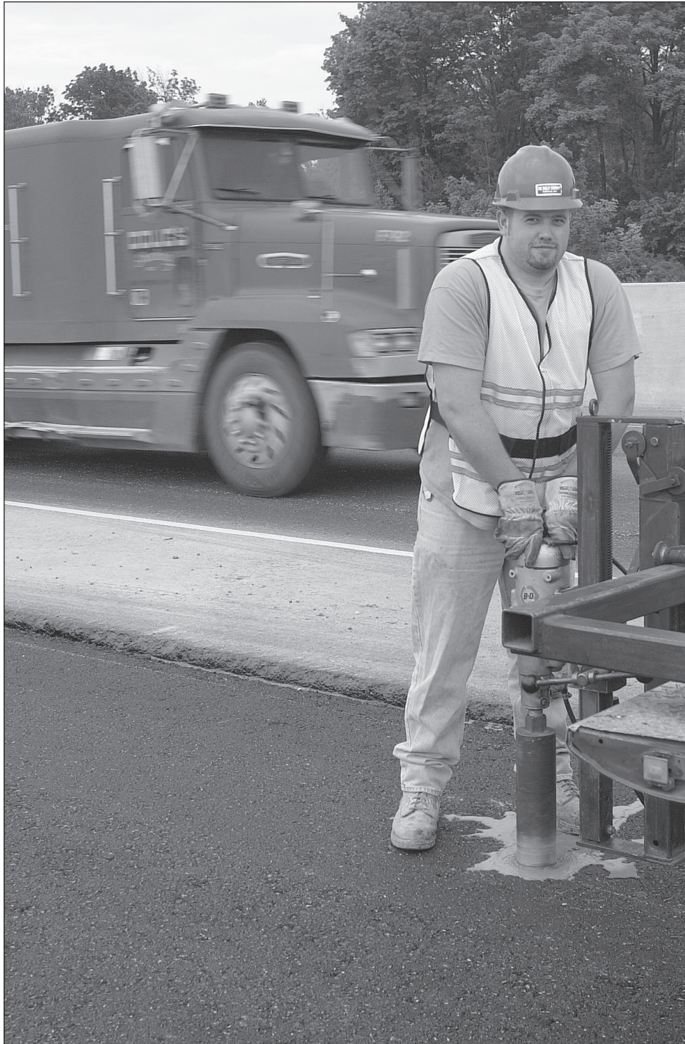
Core technician Jeff Grow of The Shelly Company samples recently installed asphalt near the I-270 and Sawmill Road interchange in northern Franklin County. The 2-inch core will be sent to an Ohio Department of Transportation laboratory and tested to determine if the asphalt pavement meets specifications. Photo by Michael D. Williams.
