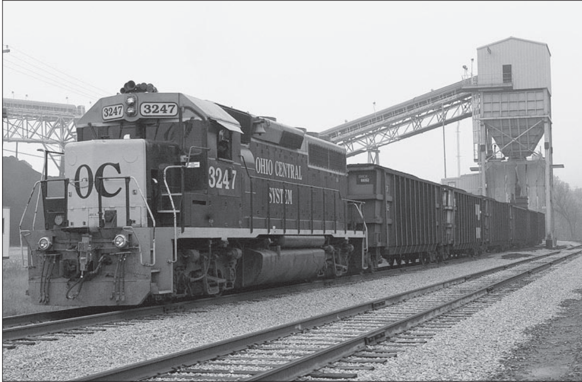
An Ohio Central unit train being loaded at the Buckingham Coal Co., Inc., mine in Athens County. The fully automated train load-out facility can load 2,300 tons of coal each hour and has a sampling system and belt scales. Photo by Michael D. Williams.
