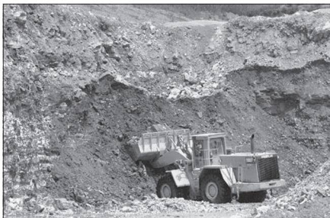
Front-end loader mining gypsum ore at the BPB-Celotex quarry in Ottawa County. The ore contains approximately 40-50 percent gypsum by weight. Photo by Michael D. Williams
