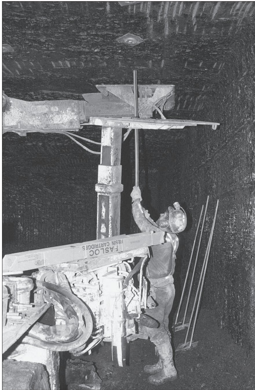
Frank Dunwoody using a Fletcher Roof Ranger II machine to install resin-type roof bolts at the underground coal mine of the Buckingham Coal Co., Inc., in Athens County. Photo by Michael D. Williams.
