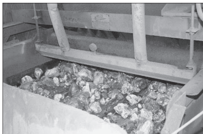
Gypsum ore before it enters the heavy-media separation system at the BPB-Celotex operation in Ottawa County. Gypsum content is improved to 80 percent by weight following heavy-media separation. Photo by Michael D. Williams
