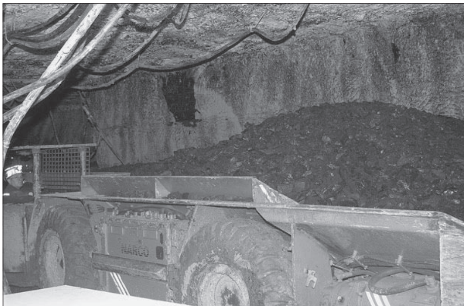
Buckingham Coal Co., Inc., employee Hillard Thacker operating a Joy 21SC-32 shuttle car at the company's underground coal mine in Athens County. The capacity of the shuttle car is 14 tons of coal. Photo by Michael D. Williams.
