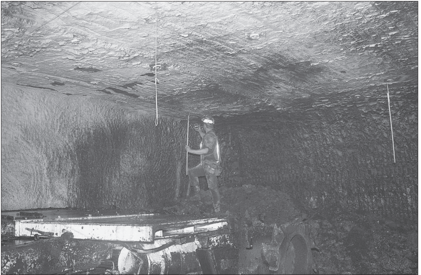
Mike Cole, continuous miner operator employed by Buckingham Coal Co., Inc., checking methane gas levels prior to mining operations at Buckingham's underground coal mine in Athens County. Note white coating of lime on walls and ceiling to minimize coal dust. Photo by Michael D. Williams.
