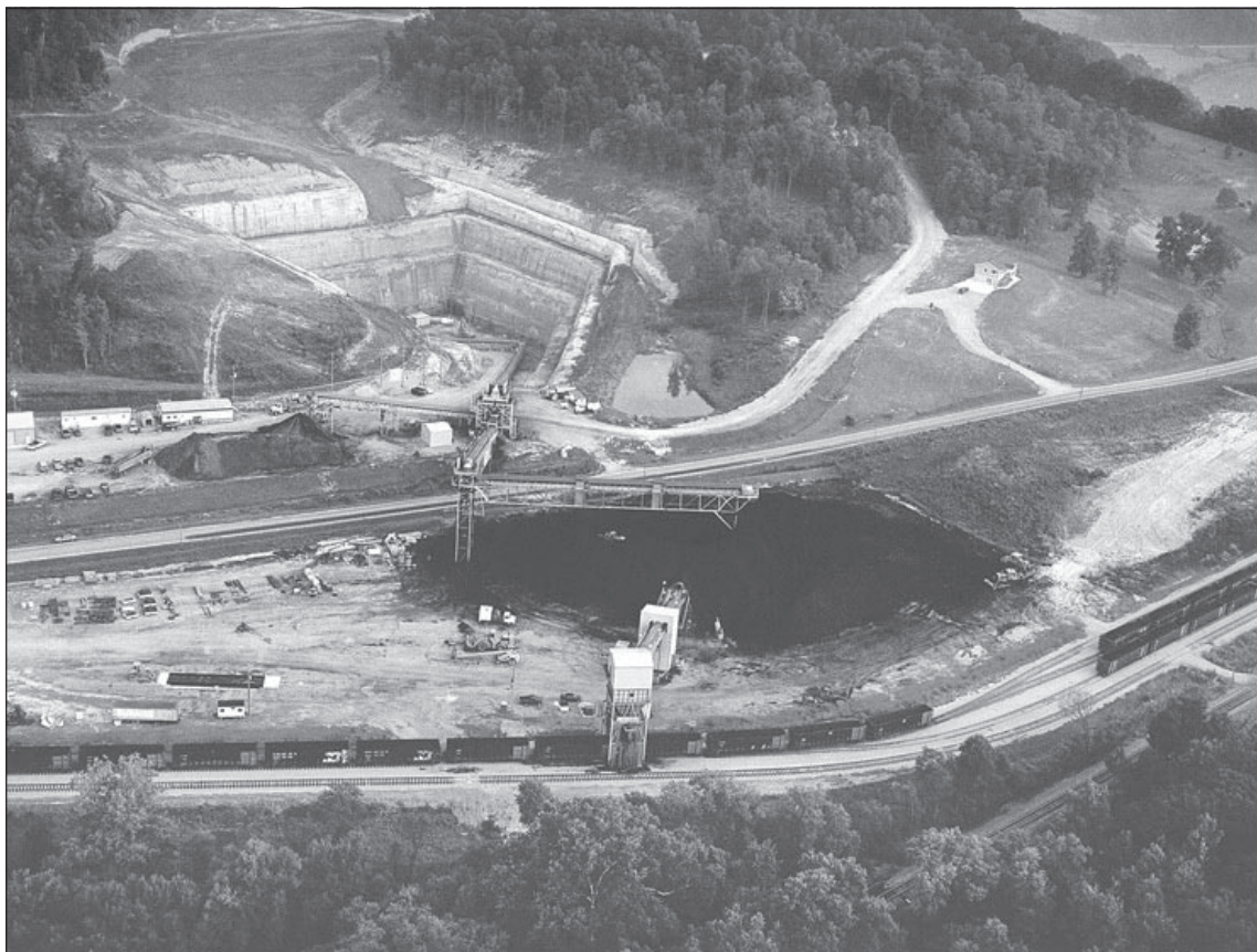
Aerial view of the surface facilities at the underground coal mine at Glouster in Athens County operated by the Buckingham Coal Co., Inc. The train load-out facility is in the foreground; offices, shops, and the entrance to the mine can be seen in the background. View is to the northwest. Photograph provided by Jeff McLean of Buckingham Coal Co., Inc.
