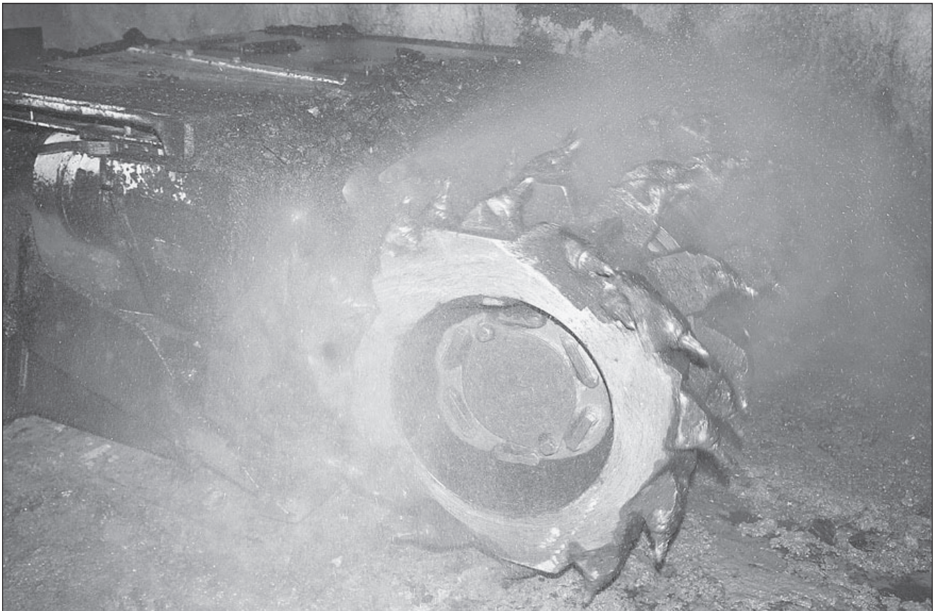
An Eimco 2810-3 continuous miner in operation at the Buckingham Coal Co., Inc., underground coal mine in Athens County. The miner is capable of mining 39 tons of coal each minute. Photo by Michael D. Williams.
