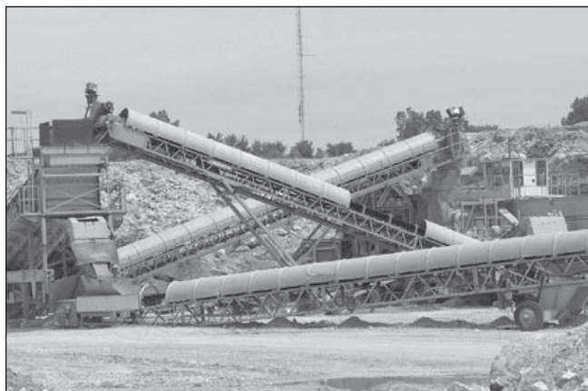
In-pit crusher and conveyor system at the BPB-Celotex gypsum quarry in Ottawa County. Photo by Michael D. Williams.
