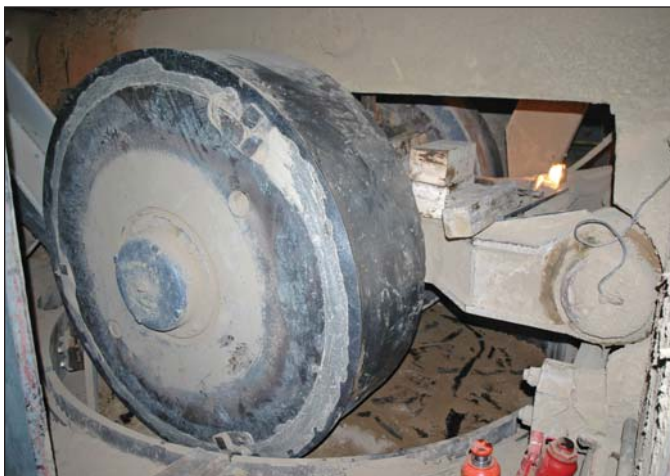
FIGURE 9. Interior view of the Clearfield Dry Pan roller-type crusher at the Ironrock/Metropolitan Brick ceramic tile plant located south of Canton, Ohio.
