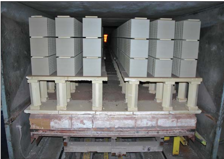
FIGURE 10. Unfired tile entering the tunnel kiln at Ironrock/Metropolitan Brick ceramic tile plant located south of Canton, Ohio.
