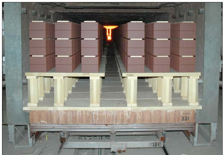
FIGURE 11. Finished tile exiting the tunnel kiln at the Ironrock/Metropolitan Brick ceramic tile plant located south of Canton, Ohio. Tiles are heated, fired to approximately 1200°C, and slowly cooled over a 24-hour period.
