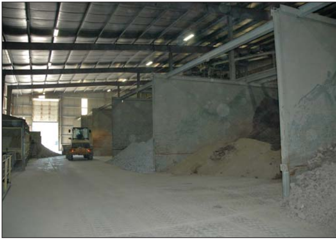
FIGURE 7. Clay and shale storage at the Ironrock/Metropolitan Brick ceramic tile plant located south of Canton, Ohio.
