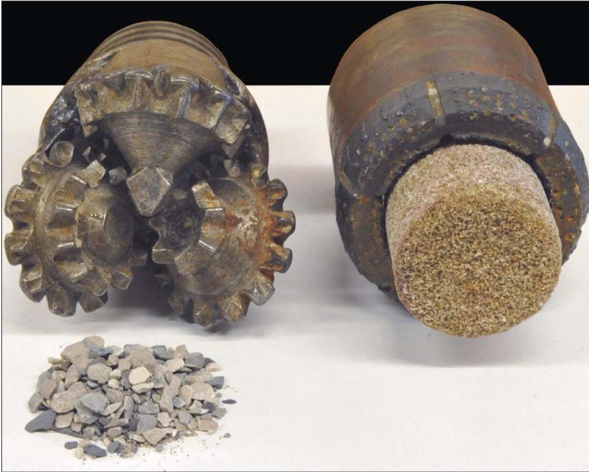
FIGURE 4.—Typical drill bits. Core drill bit with example of drilled core (right) and tri-cone drill bit with an example of well cuttings collected from a boring for an oil-and-gas well.
